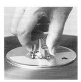
**Threading of tape:** Thread tape according to illustration below. The tape must be threaded neatly around the tape tension arm (3). Thread leading tape end onto right-hand reel and manually rotate the take-up reel in a counter-clockwise direction until the tape is locked. Tape fitted with a transparent leader should be wound forward until the start of the magnetic surface has passed the heads. Set tape counter to zero by pressing the reset button (2).
