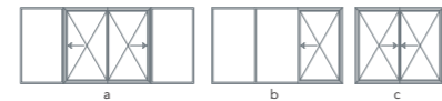
a. Sliding sash/ fixed frame 4 part b. Sliding sash/ fixed frame with side light c. Sliding sash
