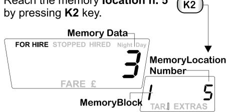
Reaching location n. 5, press **K4** key to print out the content of both Block1 and Block2. For Hire sign stops blinking and the printer will start.
