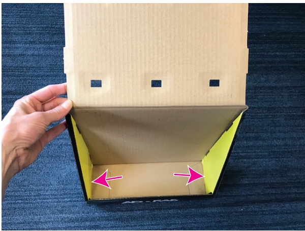
7. Secure the sides by pressing notches into the bottom holes.
