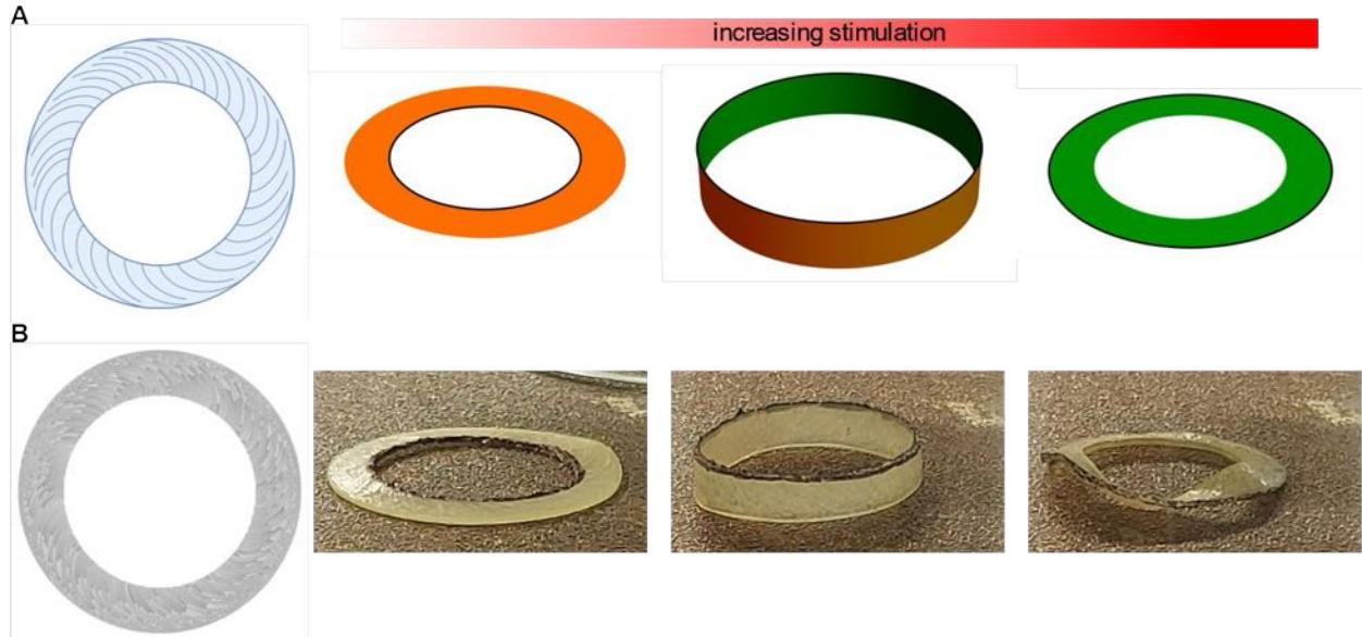
Fig. 1. Evertor director pattern as designed (A) [1], and sliced and fabricated (B). The actuation of the evertor turns the flat annulus inside out, with its original inner radius becoming the outer one.
