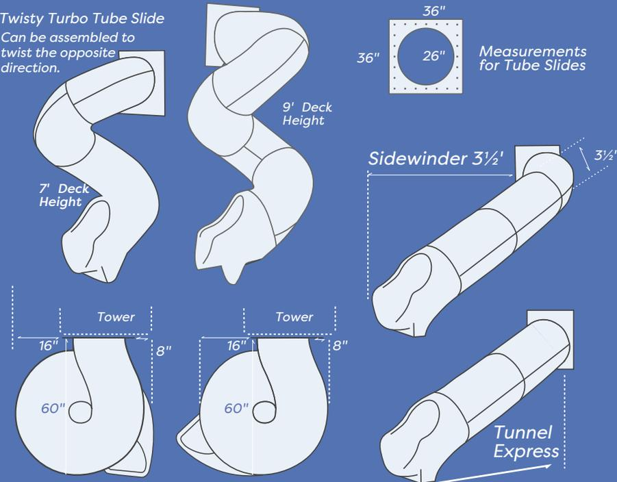
NOTE: You will need the step and slide adapter to mount a twisty turbo, extreme ripple rush slide on any 5 ft. deck.
