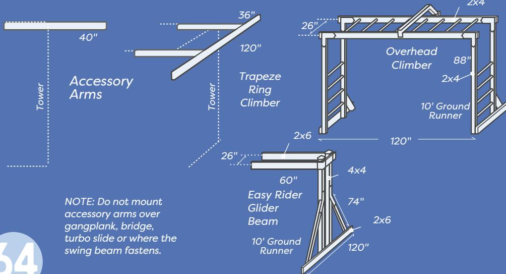
NOTE: Do not mount accessory arms over gangplank, bridge, turbo slide or where the swing beam fastens.
