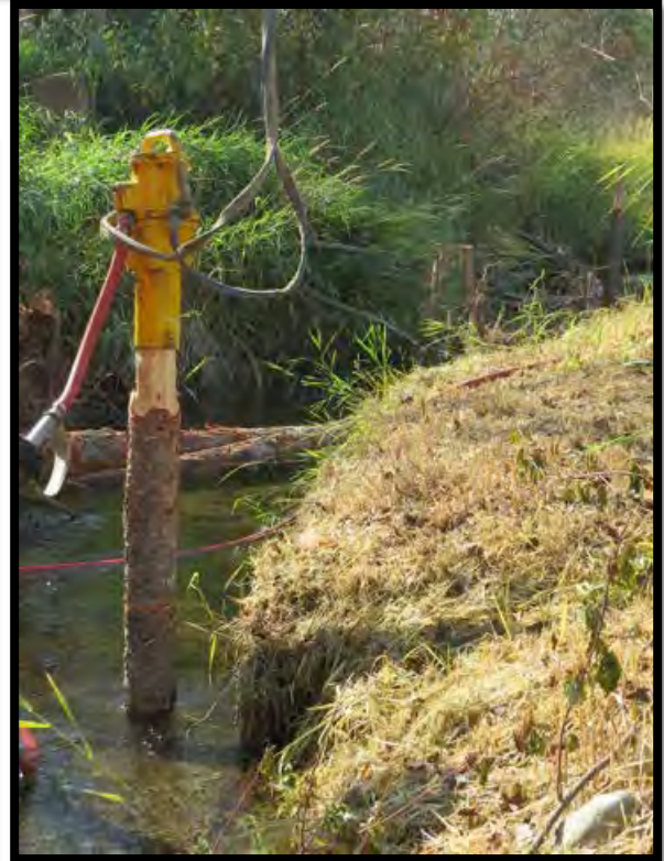
Figure 27: Hydraulic post pounder options. Options include, clockwise, starting from upper left: (a) a hand-held pounder attached to hydraulic power pack, (b) a post pounder attached to bulldozers, (c) a handheld pneumatic post pounder attached to an excavator and (d) a modified excavator with a vibrating pad. Options (a) and (b) take approximately 5 to 10 minutes per post, depending on substrate, and it can be difficult to get to the desired depth. Option (d) takes less than 1 minute per post and can drive posts as deep as needed. All pounders have a metal cylindrical cap that holds the post in place while pounding. Each option has pros and cons to consider, including cost, maximum depth the posts can be pounded, substrate type, operator strength and expertise, and the amount of likely riparian and instream disturbance. Photo credits: (a) Nick Weber, Ecological Research, (b) Mark Cookson, USFWS, (c) Peter Thamer, Siskiyou County Resource Conservation District, and (d) Julie Ashmore, Okanogan Highlands Alliance.
