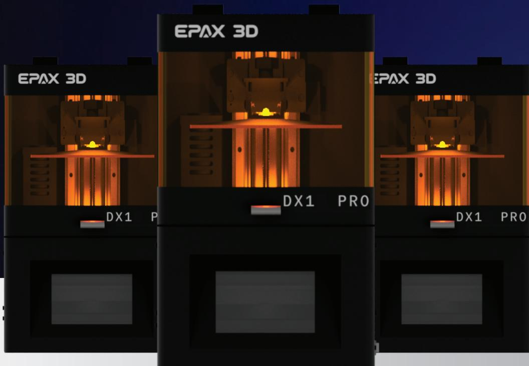
The EPAX DX1 Pro brings quick and accurate results to dental clinics using the most advanced LCD 3D printing technology in today's market. The DX-1 5.5 inch mono screen provides more print detail for dental applications where finer details are beneficial with more even distribution of the light across the entire build area.
