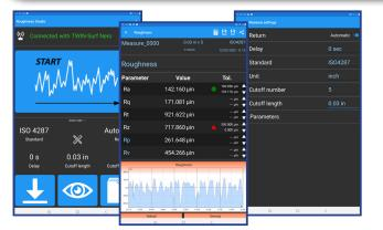
With the standard Roughness Studio APP, the instrument can be connected to an Android or Windows device and allows you to download measurement data in real time or at a later time from the internal memory of the roughness tester.
