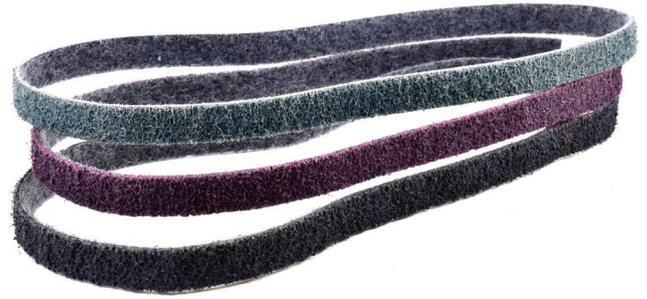
Without compromise between edge durability and flexibility, S-Flex Surface Conditioning Belts withstand critical Aerospace and General Fabrication applications requiring narrow belt operations. The semi-friable, aluminum oxide grains provide sharp cuts and consistent finishing throughout belt life and resist shedding or chunking due to their micro-fracture properties.
