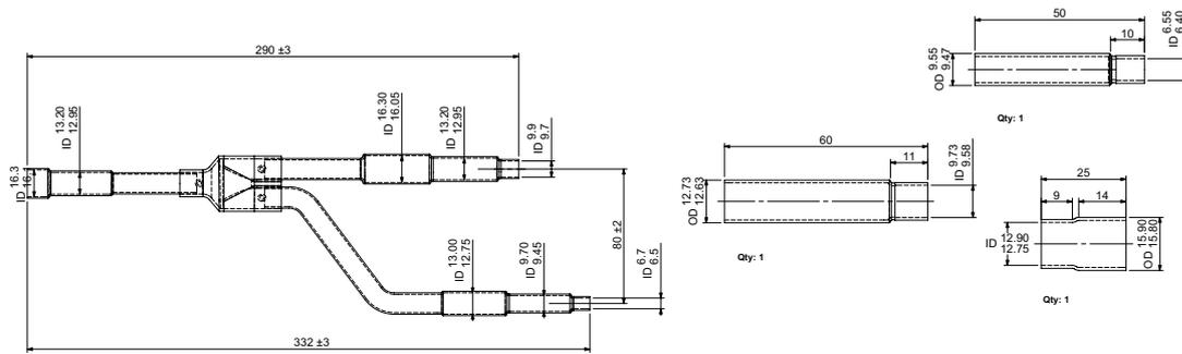
All measurements are in mm. Size of connection points on each part shown are inside diameters of piping.
