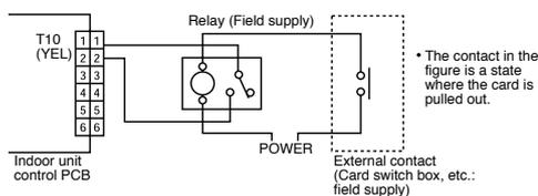
NOTE: The wire length from indoor unit to the Relay must be within 2.0m
