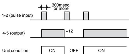
NOTE: The wire length from indoor unit to the Relay must be within 2.0m. Pulse signal changeable to static with JP cutting. (Refer to JP001)
