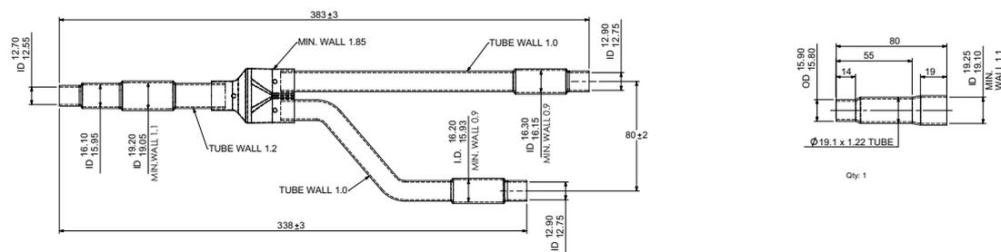
All measurements are in mm. Size of connection points on each part shown are inside diameters of piping.
