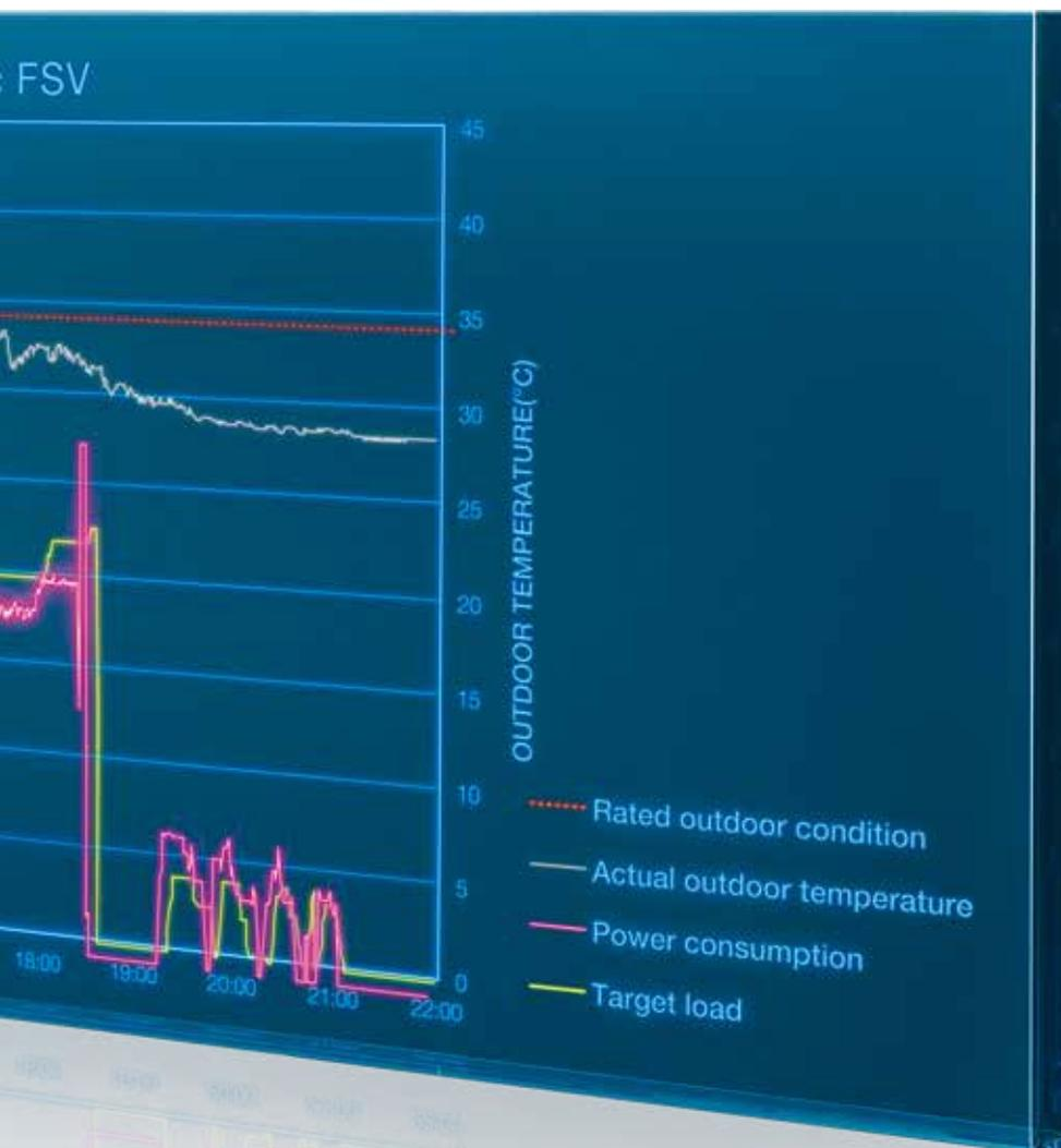
**Set temperature maintained with minimum load operation**
