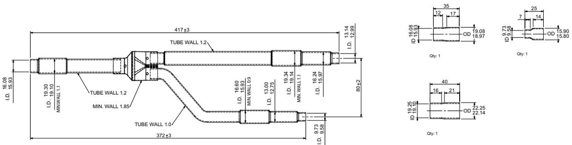
All measurements are in mm. Size of connection points on each part shown are inside diameters of piping.
