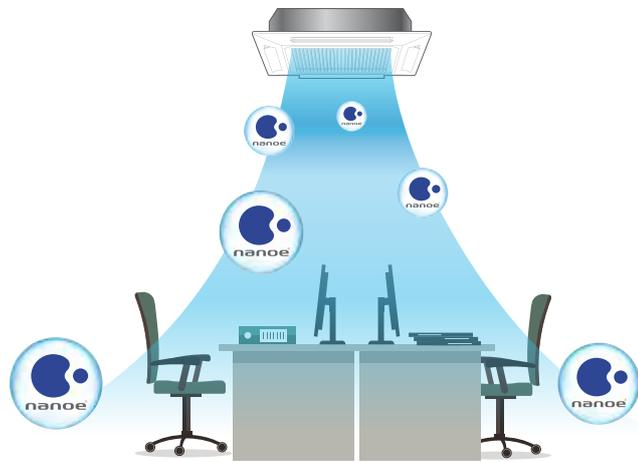
nanoe particles are discharged from a single port, then carried and dispersed on the air conditioner's airflow.
