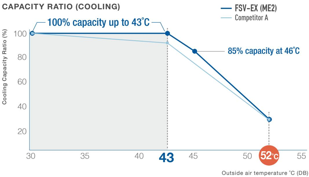
Test Conditions: 33.5kW model, IU/OU capacity ratio: 100%, Indoor Condition: 27°C[DB]/19°C[WB]
