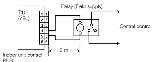
NOTE: The wire length from indoor unit to the Relay must be within 2.0m. Pulse signal changeable to static with JP cutting. (Refer to JP001)
