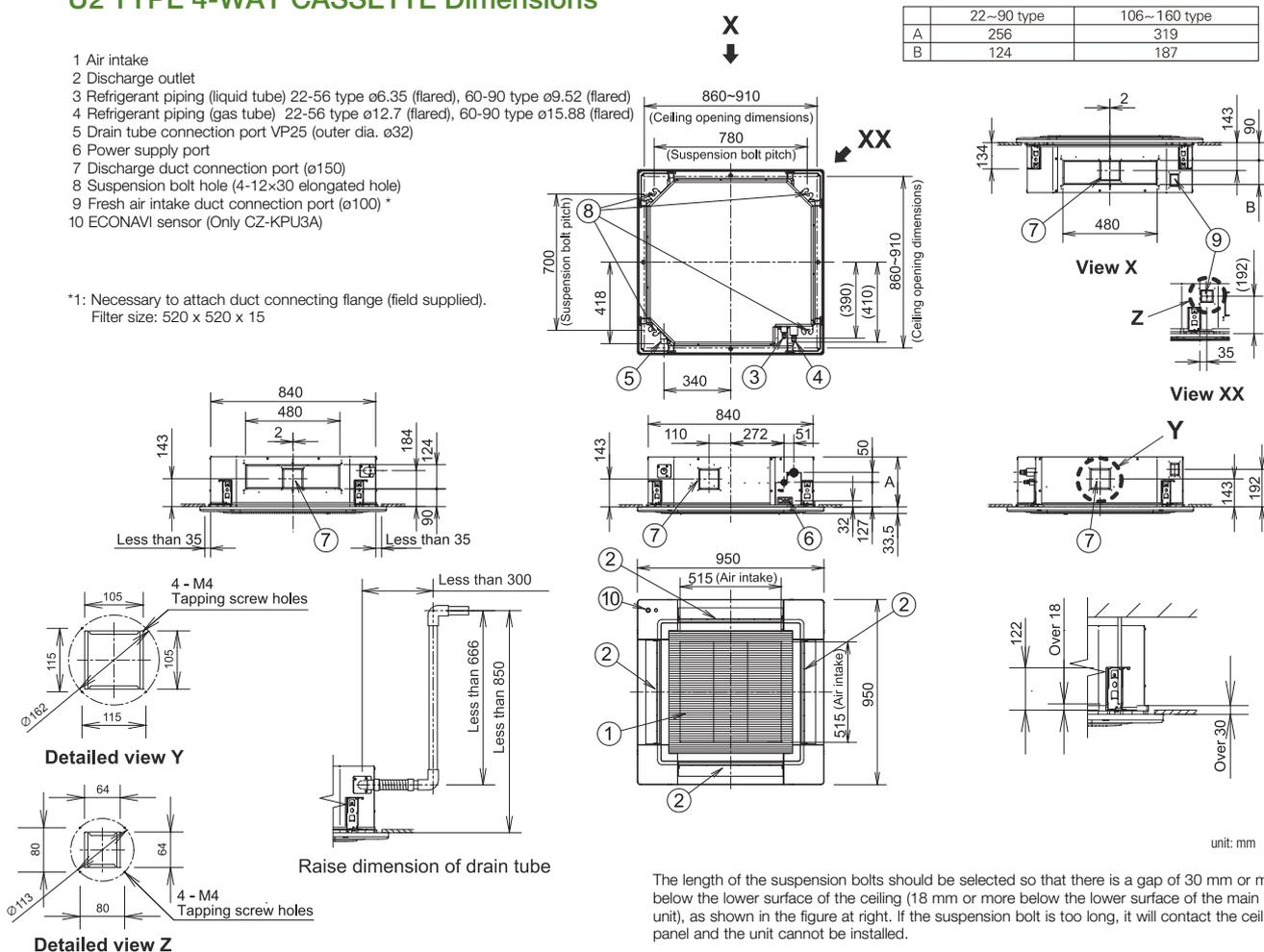
The length of the suspension bolts should be selected so that there is a gap of 30 mm or more below the lower surface of the ceiling (18 mm or more below the lower surface of the main unit), as shown in the figure at right. If the suspension bolt is too long, it will contact the ceiling panel and the unit cannot be installed.
