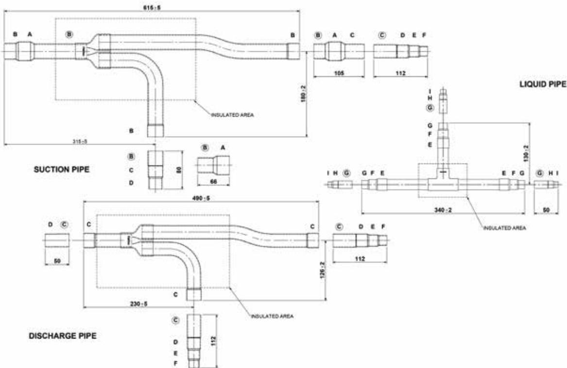
All measurements are in mm. Size of connection points on each part shown are inside diameters of piping.
