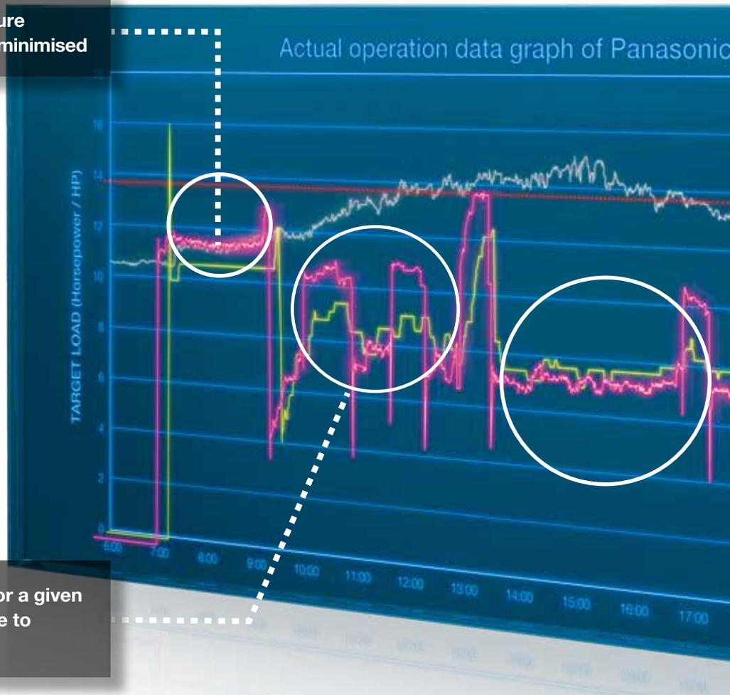
Load increased as required for a given outdoor temperature increase to maintain the set temperature
