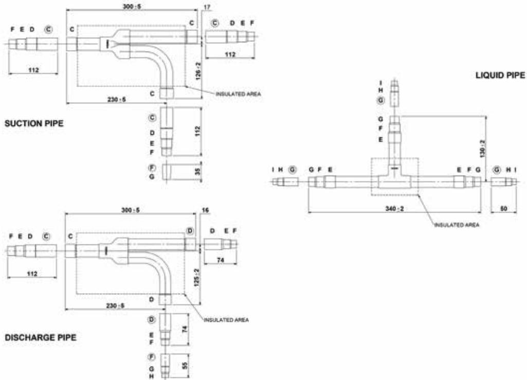
All measurements are in mm. Size of connection points on each part shown are inside diameters of piping.
