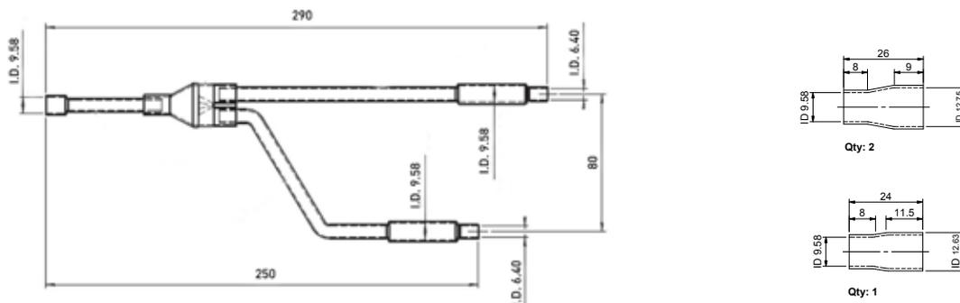
All measurements are in mm. Size of connection points on each part shown are inside diameters of piping.
