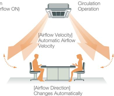
Furthermore, with 2 indoor units installed, when the absence of people is detected while the indirect Airflow setting is ON, circulation operation is automatically activated.
