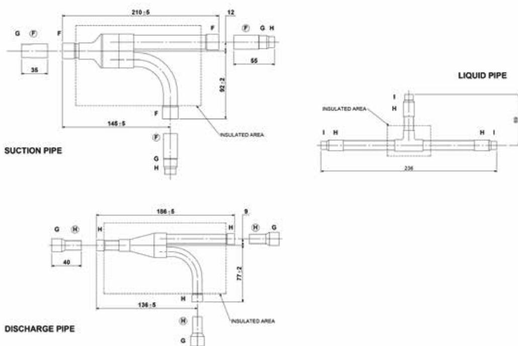
All measurements are in mm. Size of connection points on each part shown are inside diameters of piping.
