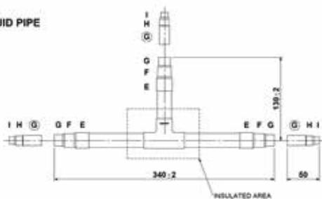
All measurements are in mm. Size of connection points on each part shown are inside diameters of piping.
