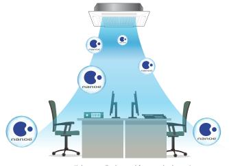
nance particles are discharged from a single port, then carried and dispersed on the air conditioner's airflow.
