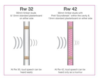
Rw is the weighted sound reduction in dB and it describes the airborne sound insulating power of a building element.
