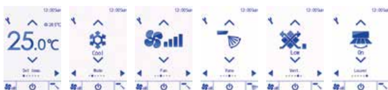
Temp. Setting Operation Mode Fan Speed Vane Control Ventilation Louver Control
