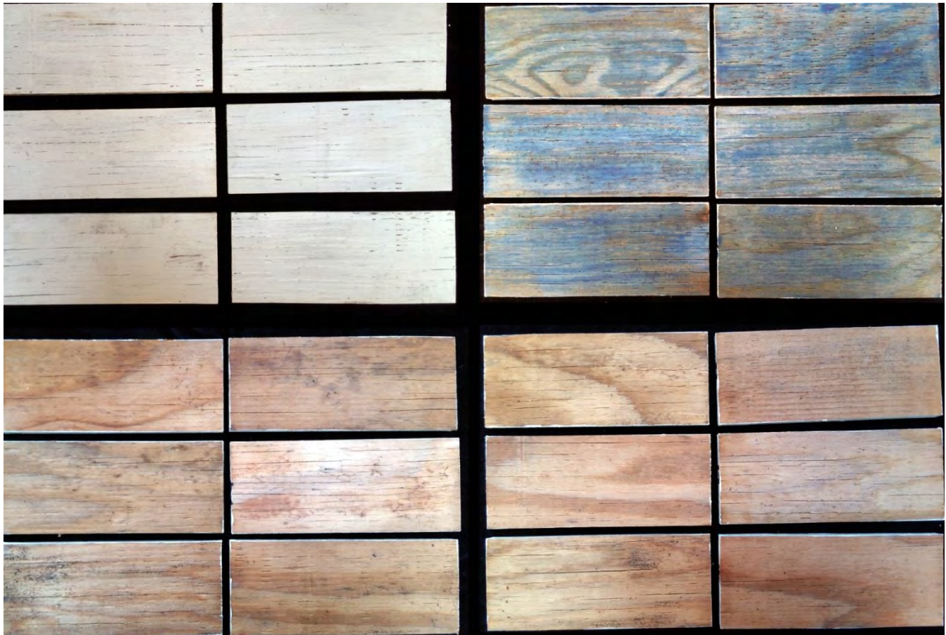
Figure 4. Samples after 12 weeks' exposure. Top left: Product D remains white, but appears aged and a bit greyer/yellower and clear of any new mould growth. Top right: Product B has some loss of blue colour intensity, when wet the wood grain and stain below become more visually pronounced. Bottom left: Product C-treated samples, both new and previous mould visible. Bottom right: sample treated with Product A does not mask previous mould or stain while some new growth was inhibited.
