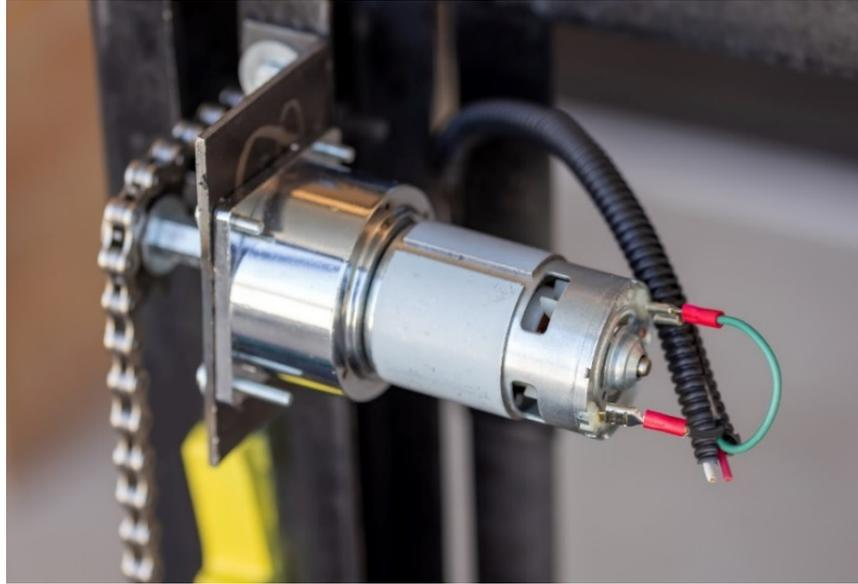
***Figure 90: Lifting motor mount***
