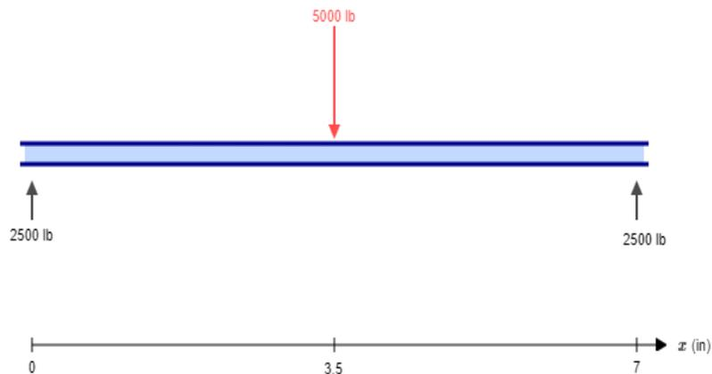
**Figure 40: Free Body Diagram of a simply supported beam.**
