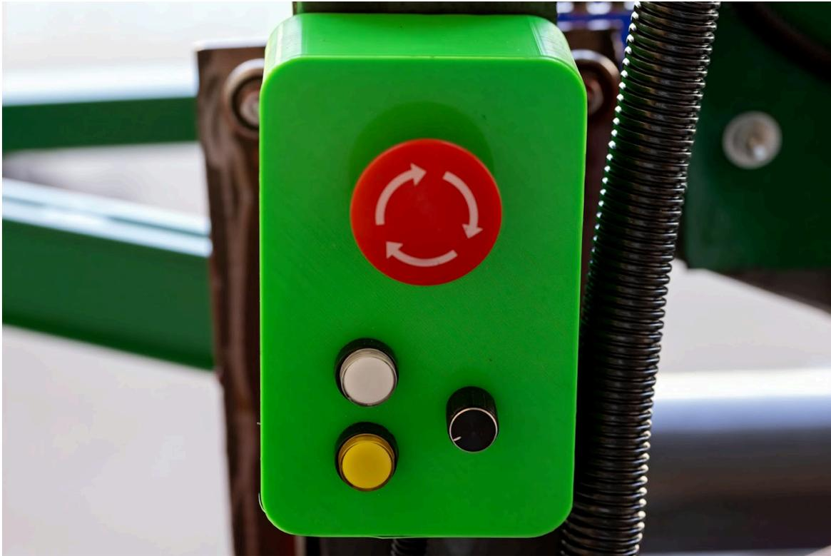
*Figure 101: VFD and limit switch remote control*
