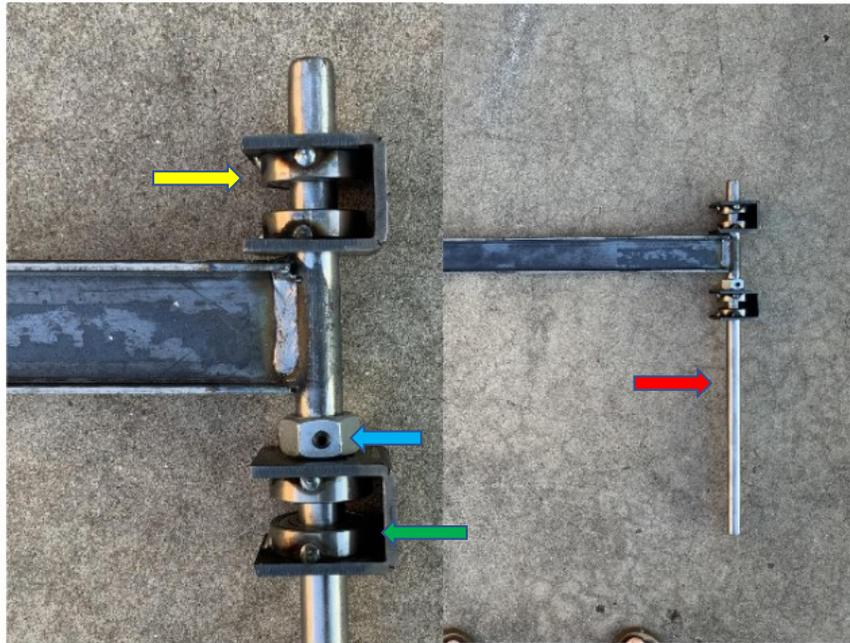
***Figure 87: Jib Pivoting Assembly***
