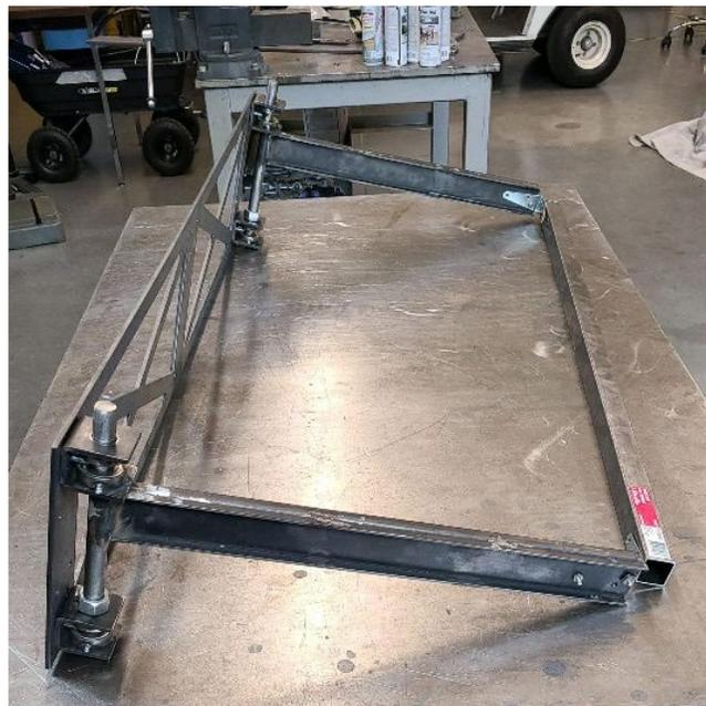
***Figure 88: Weld head track connected to the jibs***
