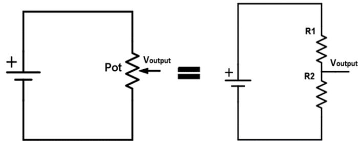
**Figure 74: Potentiometer Schematic [23]**
