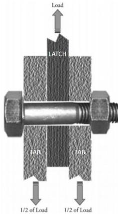
**Figure 46: Forces acting on the bolt [15]**
