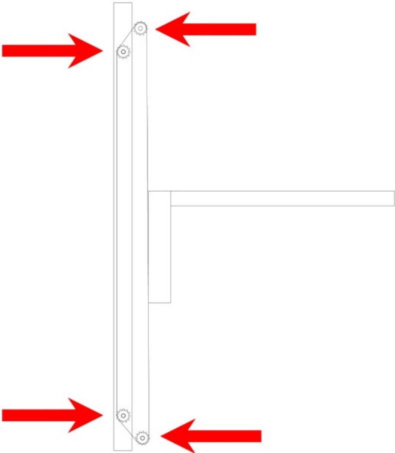
**Figure 36: Hoist chain sprockets**
