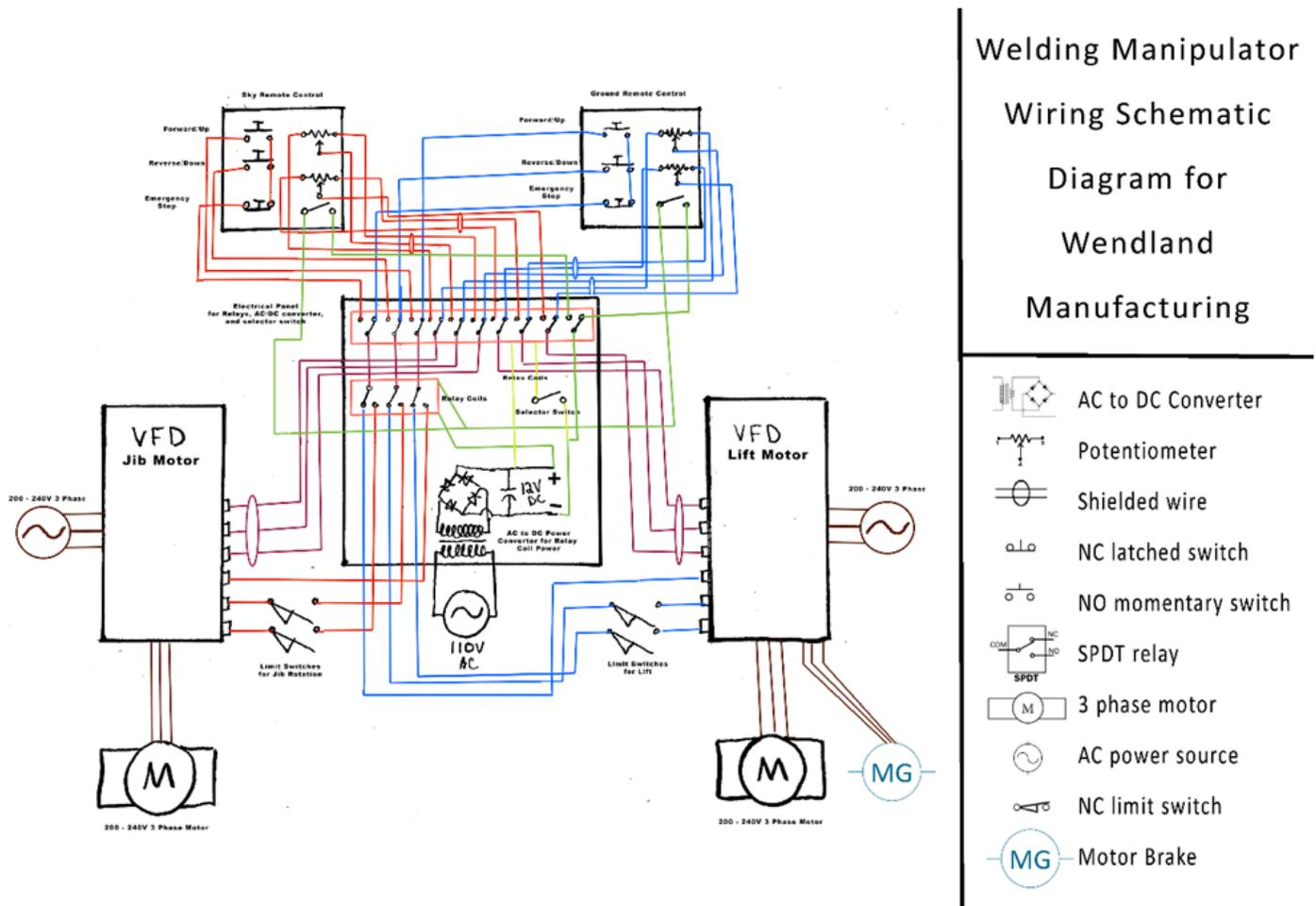
**Figure 76: Wiring Diagram for Weld Head Manipulator**
