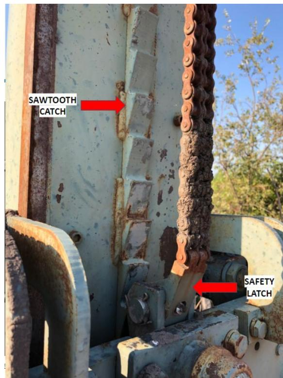
*Figure 23: Weld manipulator safety latch example.*
