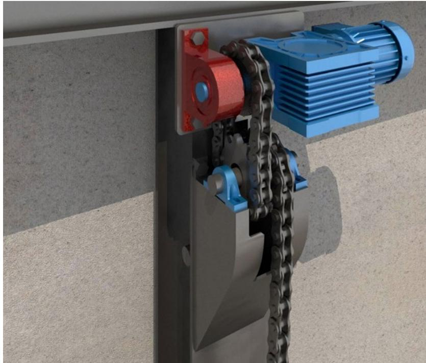
***Figure 17: Lifting Shaft Assembly Platform***
