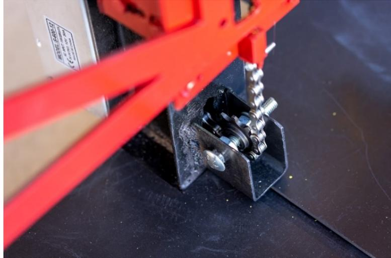
*Figure 93: Bottom sprocket mount*
