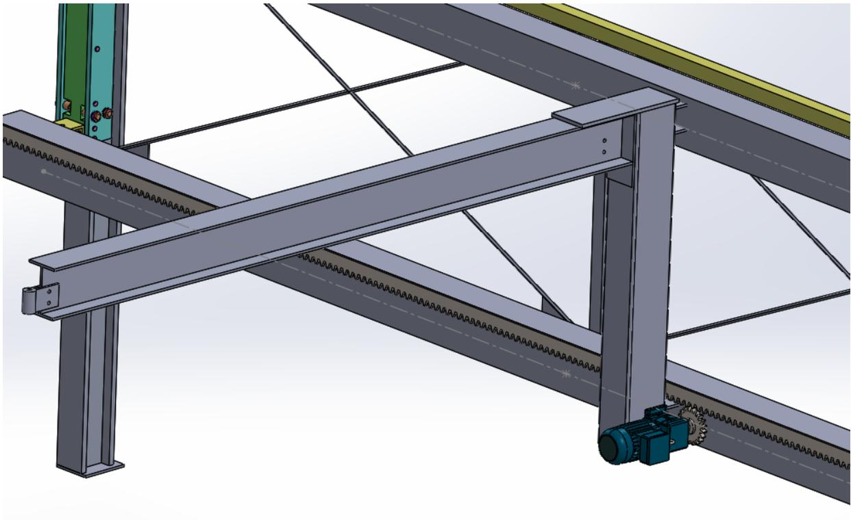
***Figure 55: Option2 - Rack and Pinion***
