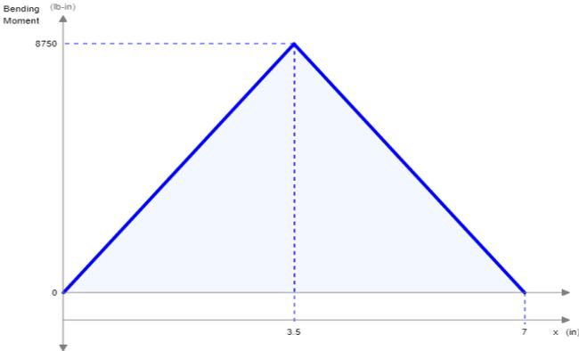
**Figure 42: Bending moment diagram of the shaft.**
