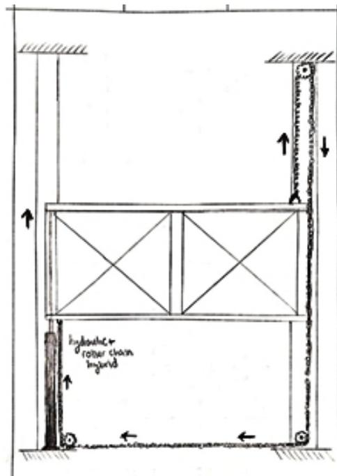
***Figure 13: Option 4 - Hydraulic piston with a chain and sprocket system***
