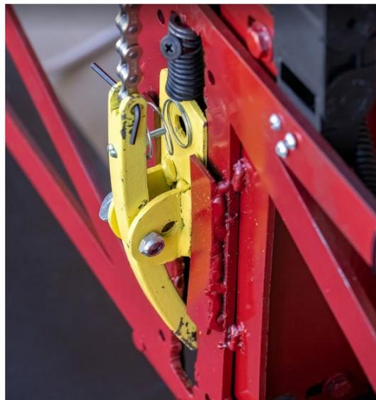
*Figure 94: Safety latch mechanism*
