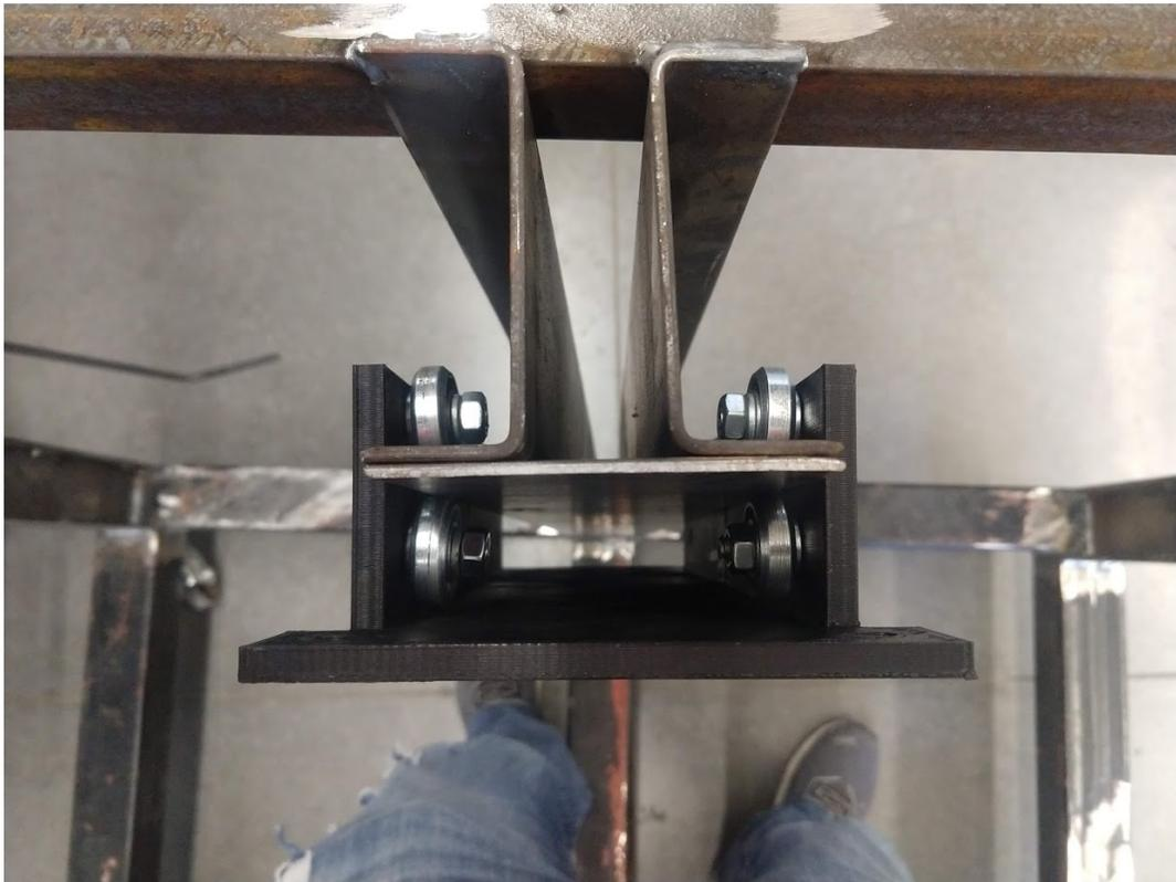
*Figure 82: Cross-section of the center built-up column*
