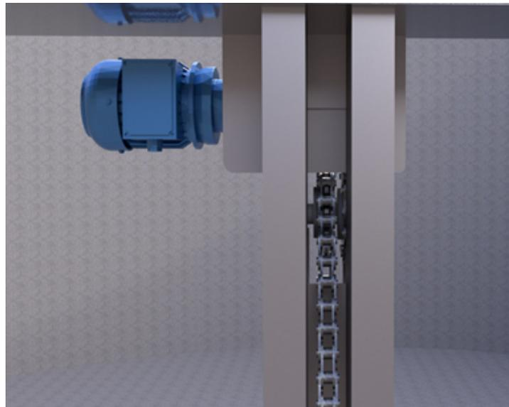
***Figure 15: Backside of center column with chain located within***
