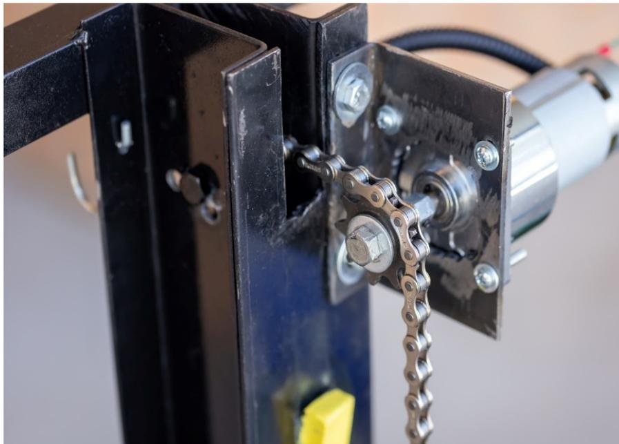
***Figure 91: Sprocket and shaft adapter***
