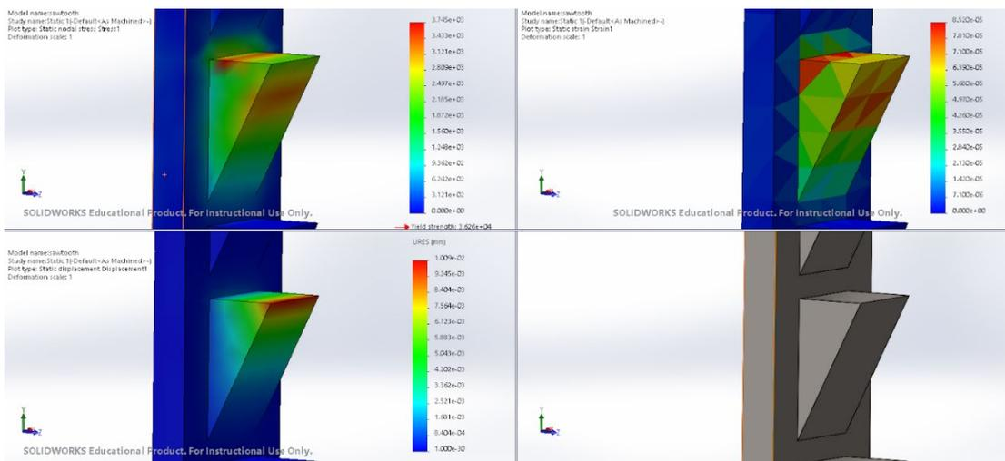
**Figure 49: FEA of the Sawtooth catch**
