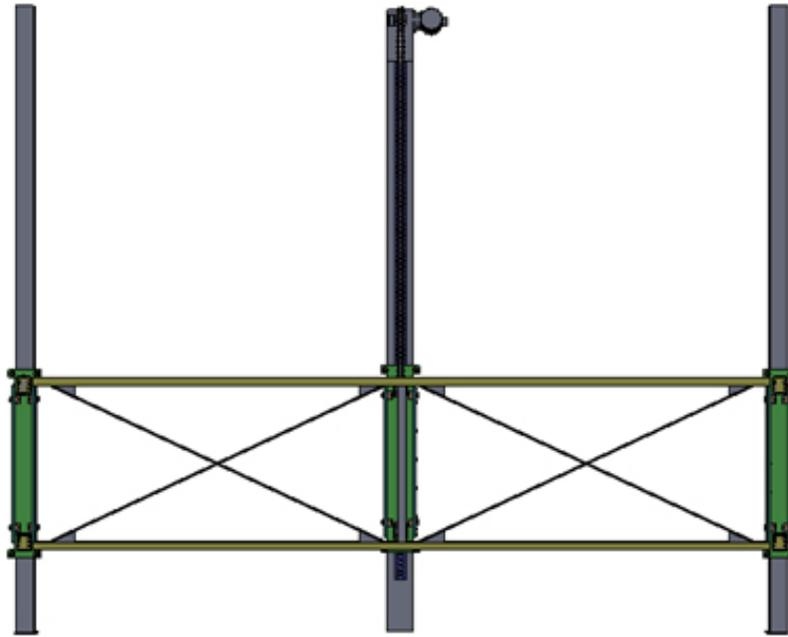
***Figure 14: Option 5 - Motor, chain, and sprocket combination***
