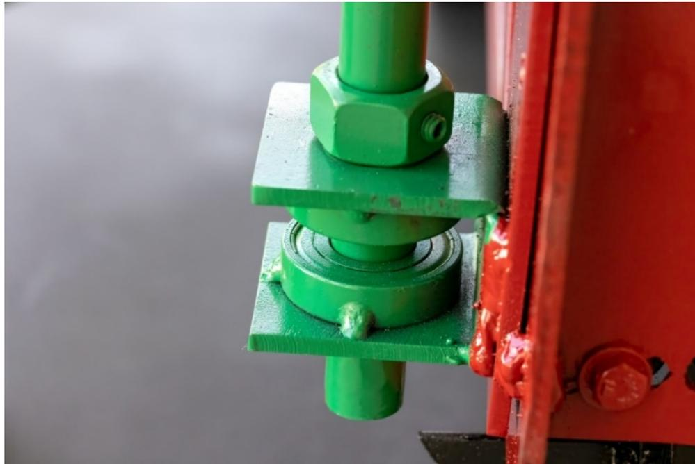
*Figure 89: Jib welded to the carriage*
