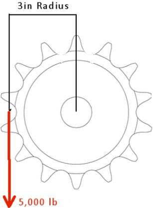
Figure 38: Sprocket torque and radius
