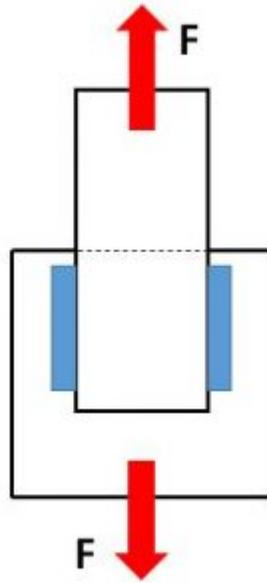
*Figure 29: Fillet welds loaded in shear [29]*
