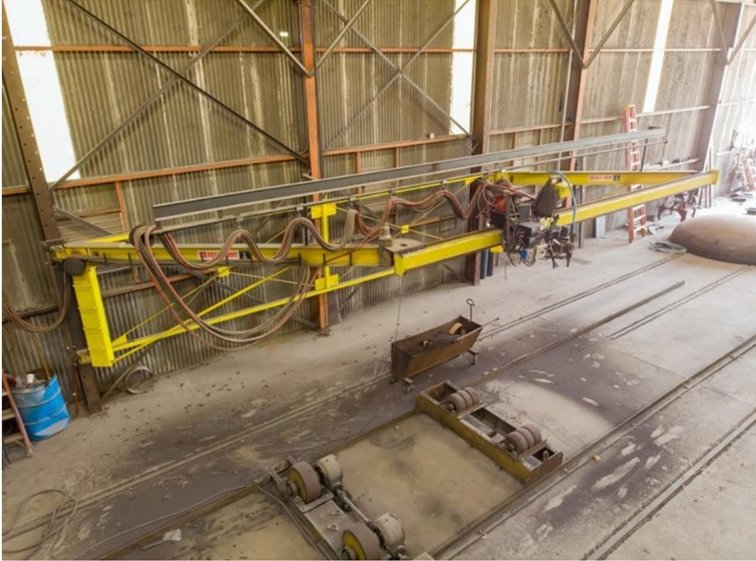
***Figure 1: Existing welding manipulator at Wendland Manufacturing***
