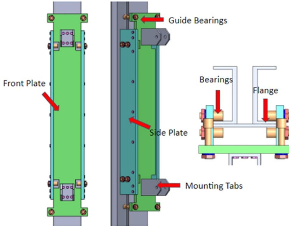
***Figure 27: Sled Design on existing Machine***
