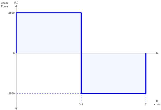
**Figure 41: Shear diagram of the shaft.**
