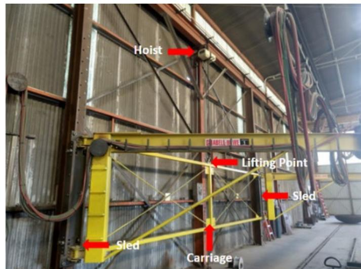
*Figure 3: Current Machine Hoist and other components*
