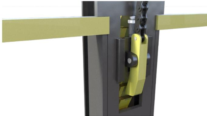
*Figure 21: Option 3: Cad model of weight driven safety latch*
