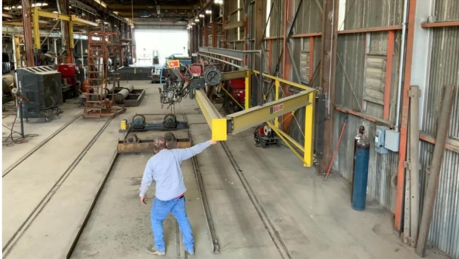
***Figure 52: Pivoting motion of the jib assembly***
