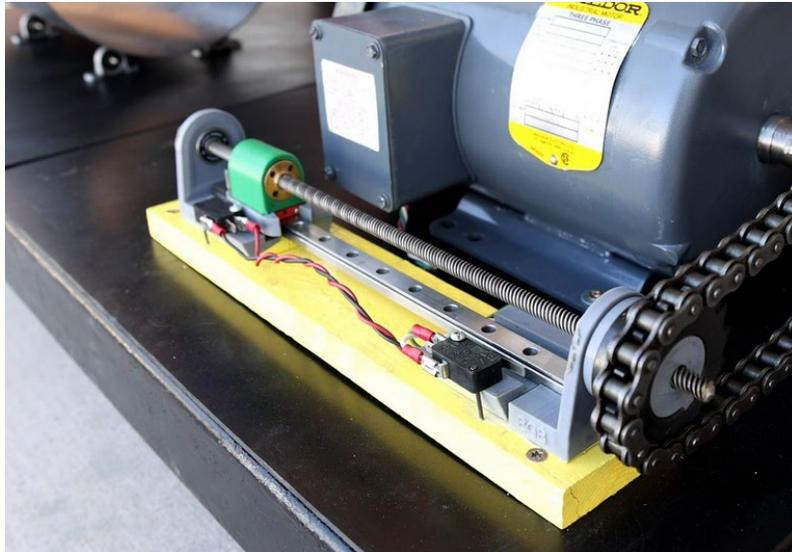
*Figure 98: Limit switch assembly*
