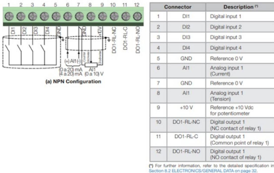
Figure 67: VFD Control wire inputs [6]
