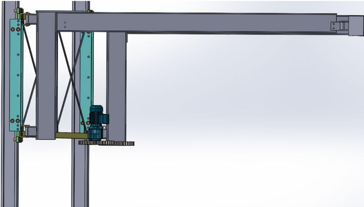
***Figure 56: Option 3 - Chain drive with motor and sprocket***
