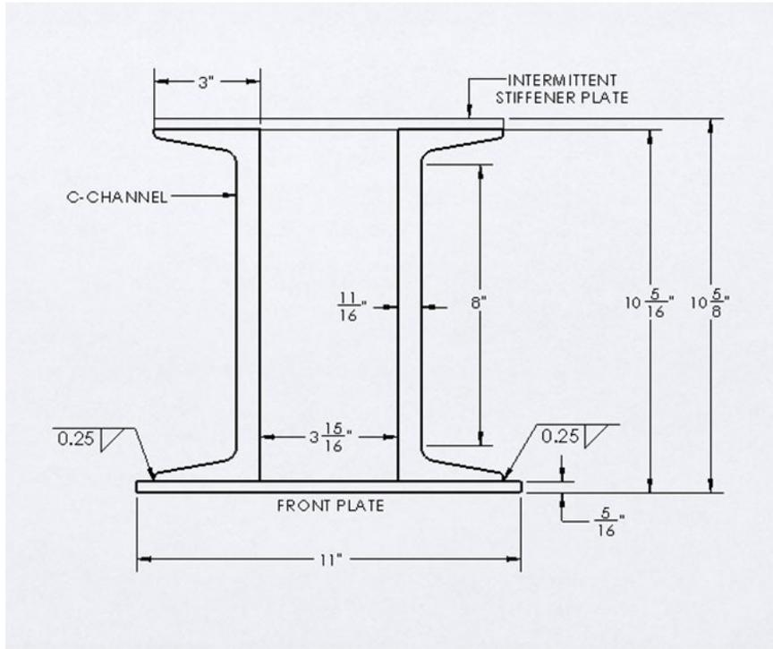
**Figure 16 : CAD model and dimensions of the built-up column**
