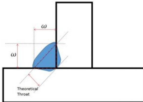
***Figure 30: Throat weld diagram[29]***
