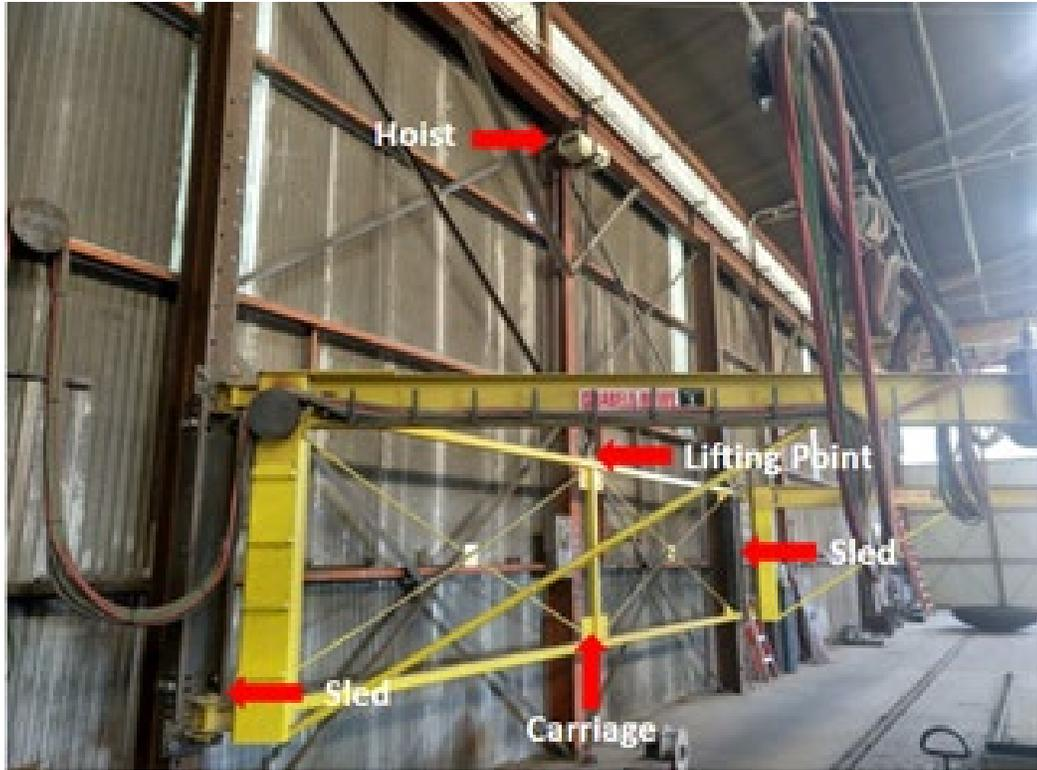
*Figure 2: Machine Components*
