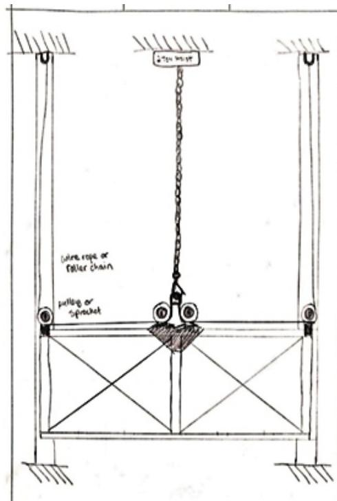
***Figure 10: Option 1-Mechanical advantage pulley system***
