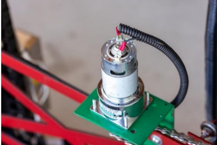
*Figure 95: 12V motor mounted using the mounting bracket*
