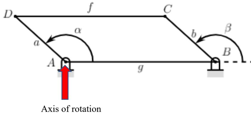
**Figure 53: Axis of rotation for the moment of inertia analysis**
