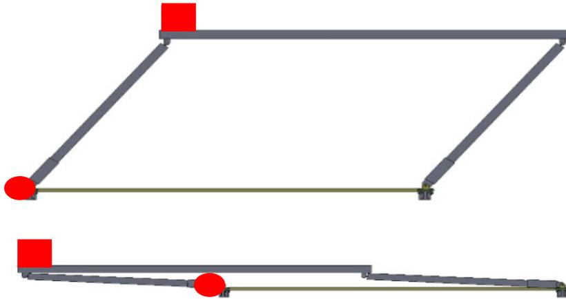
**Figure 61: Realistic weld head positioning during movement**
