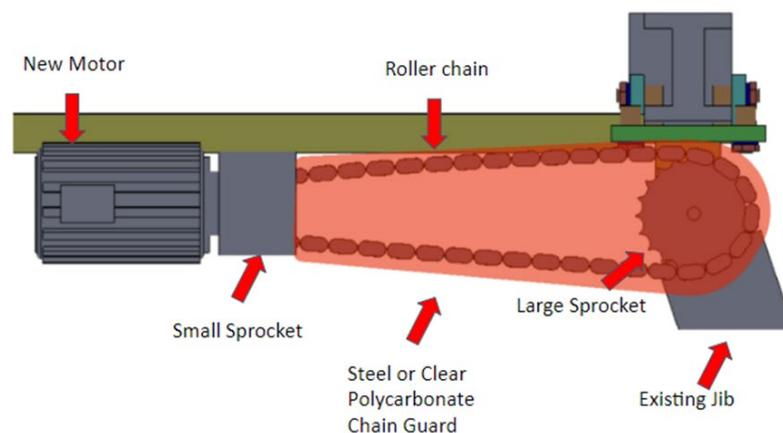
***Figure 62: Final Jib rotation assembly design***
