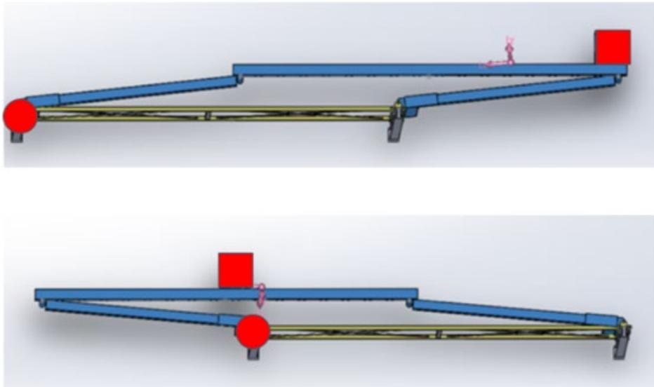
***Figure 60: Extreme positioning of the weld head from the axis of rotation***
