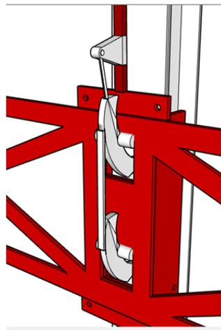
***Figure 20: Option 2-Tension cable, double latch safety mechanism.***
