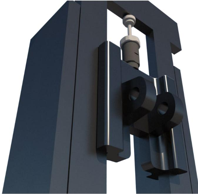
*Figure 26: CAD model of Safety latch sliding mounting plate*
