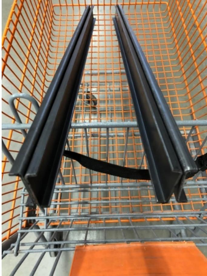
***Figure 86: C-channel sections used to fabricate the jibs***
