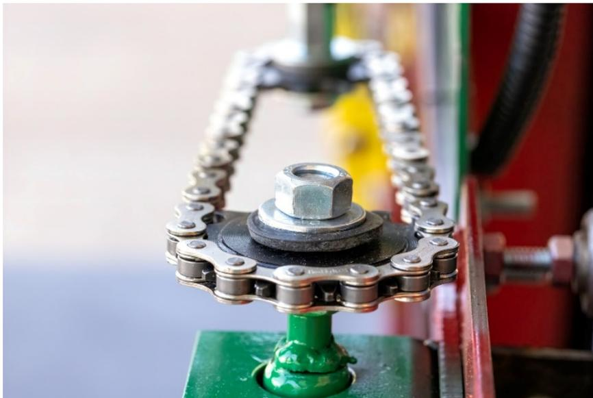
*Figure 96: Stationary sprocket for the jib motor*
