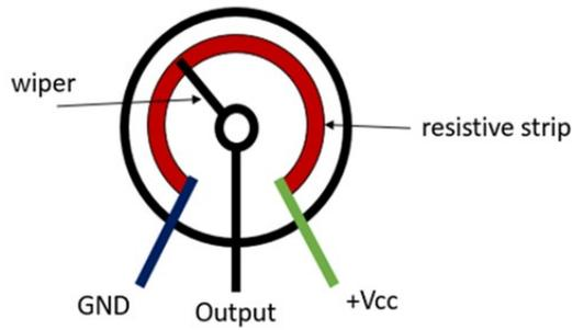
**Figure 73: Potentiometer resistive strip [23]**
