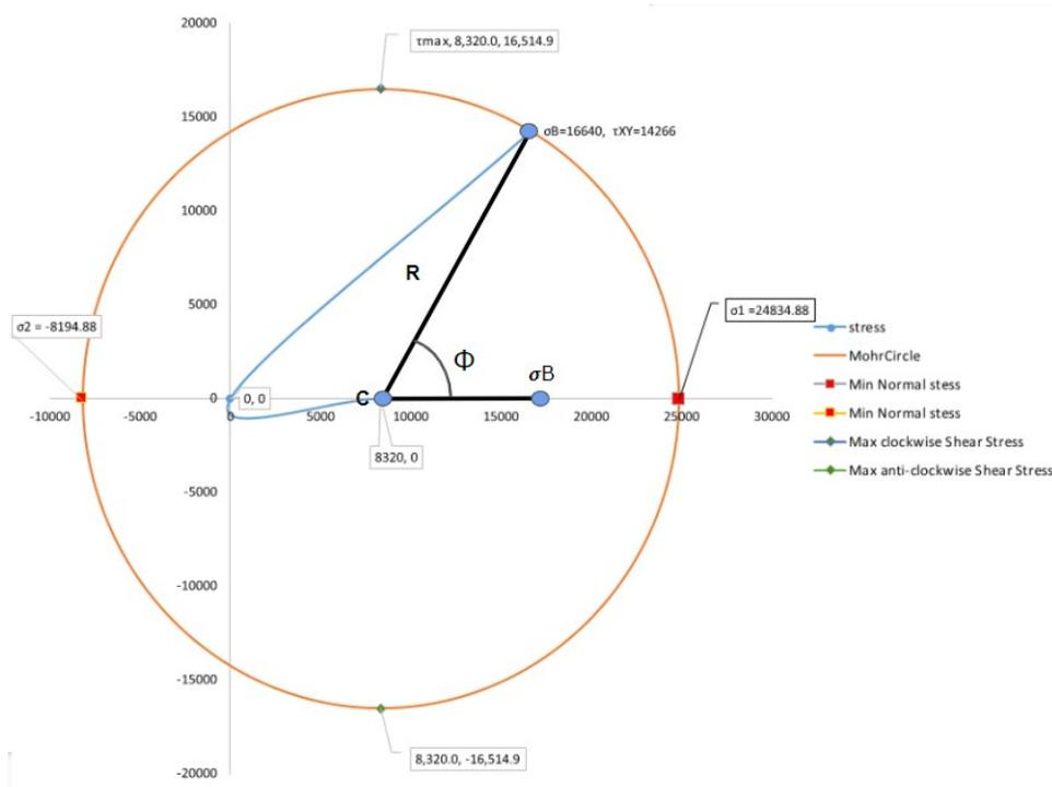
**Figure 43: Mohr's circle for maximum bending and torsional stress.**
