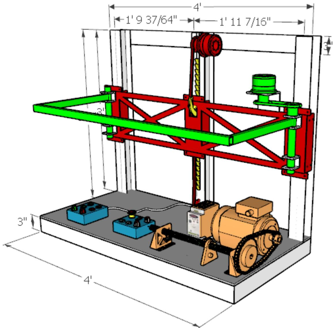
*Figure 80: Full prototype model where the red denotes the lifting mechanism, green denotes the jib rotation mechanism, yellow denotes the safety latch mechanism, and orange denotes the limit switch enclosure and the VFD*
