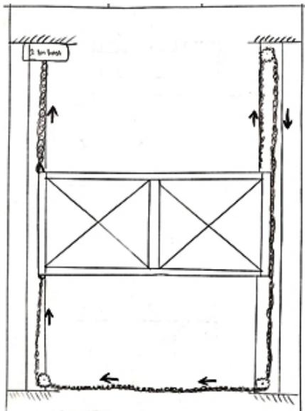
**Figure 12: Option 3 - Hoist, chain, and sprocket combination.**
