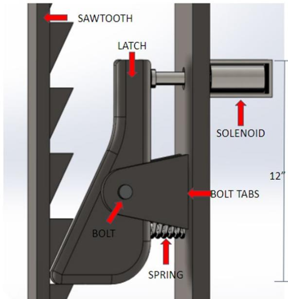
***Figure 19: Option 1-Solenoid Safety latch***
