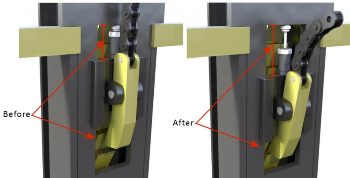
***Figure 25: CAD model before and after a chain break***
