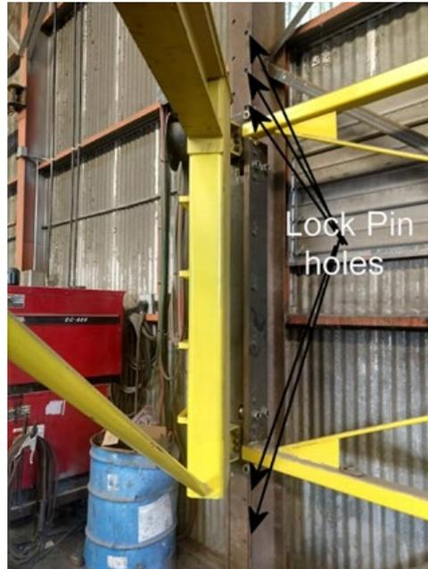
***Figure 18: Locking Pin Holes in the Column***
