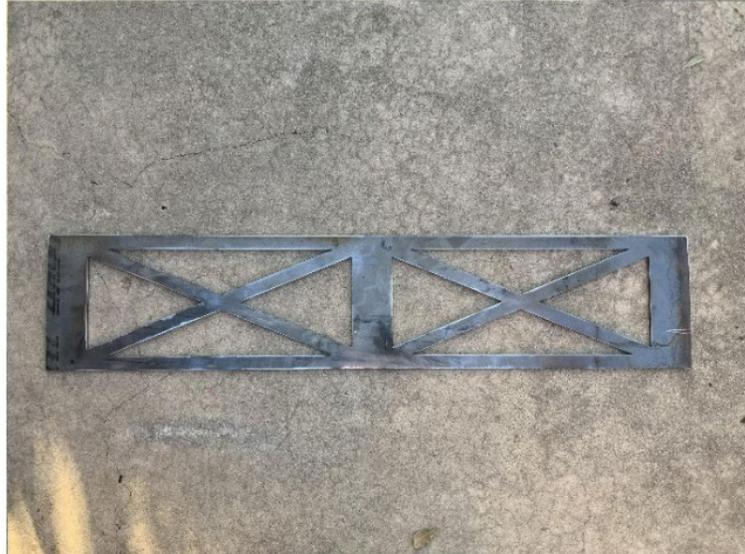
***Figure 83: CNC cut carriage frame***
