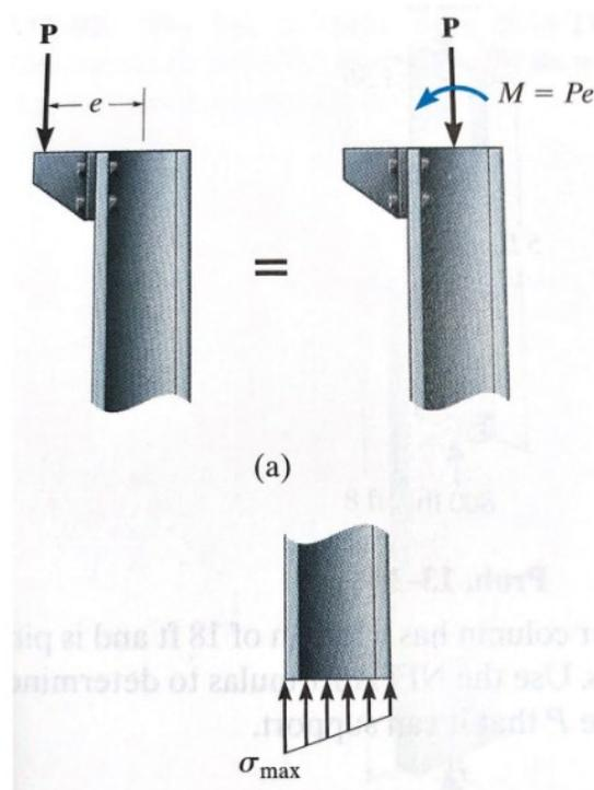
**Figure 28: Example of eccentric loading on a column [21]**
