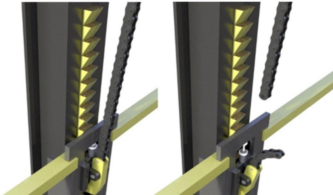
*Figure 24: Sawtooth Latch System*
