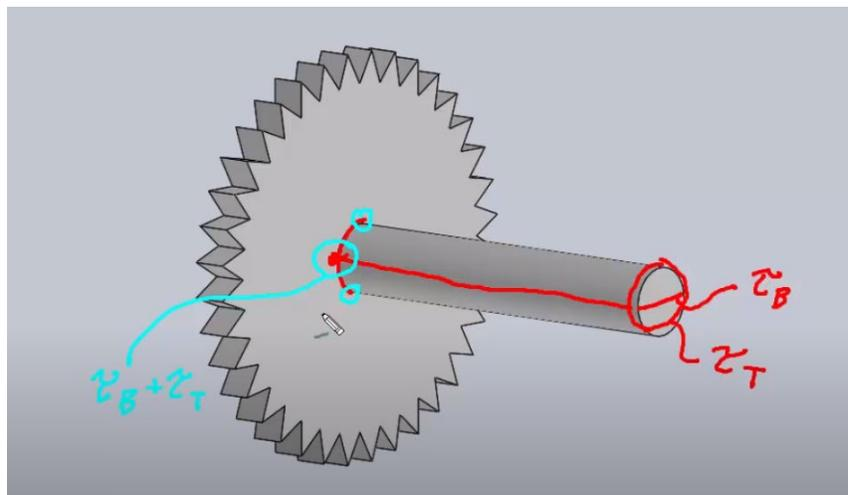
**Figure 37: Sprocket and shaft bending and torsional stresses [15]**
