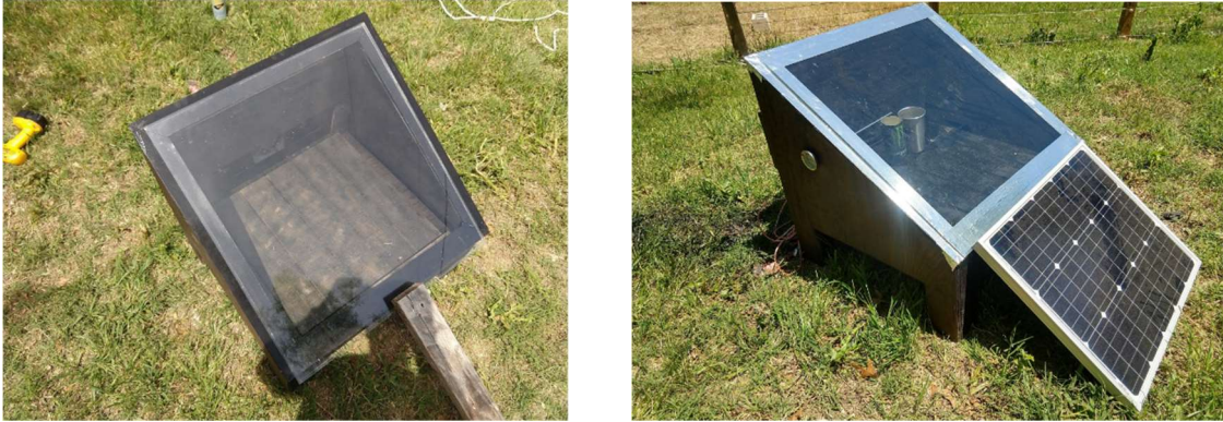
Figure 4: a) Solar Oven with Glass [left] b) Solar Oven with Solar Panel [right]
