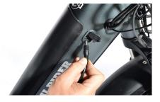
For the battery located behind the seat post, locate the charging port and plug in.
