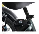
After adjusting, tighten the quick release lever.
