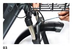
Tighten the screws to secure the mudguard.
