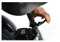
**03**Adjust the seat height to the comfortable position.
