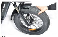
Align the front wheel with the front fork dropouts.
