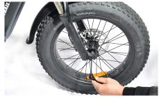
Insert the quick-release skewer into the front wheel.
