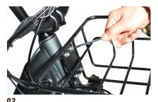
Tighten the screws using tools
