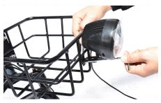
Tighten the screws to secure the front headlight.
