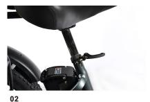
Align the seat with the seat post hole and place the seat.
