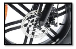
3. It is important to align the disc brake rotor with the caliper.
