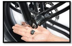
Insert the front wheel stud bolt through the front wheel center shaft, starting on the side with the disc brake.
