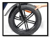
Remove the plastic protector attached on the front fork and line up the front wheel into the front fork mount.
