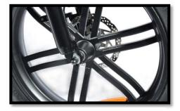
Put the front wheel screw covers on both ends of the front wheel stud bolt.
