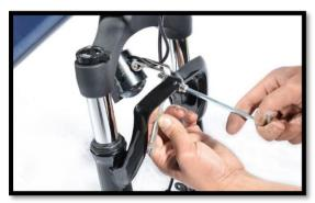
2. Install the light on the support bracket, located on the fork of the front tire.
