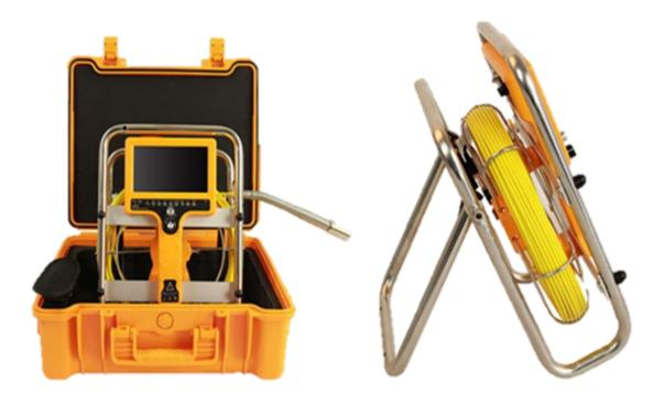
The RVI PC is a rugged Pipe Camera with a 5mm diameter fiberglass rod, 20 meter to 35 meter customizable lengths and interchangeable camera heads up to 28mm in diameter. Includes 12 levels of LED light control and a 7" monitor ready for video/ audio recording or still images. Equipment is enclosed in heavy duty ABS case.
