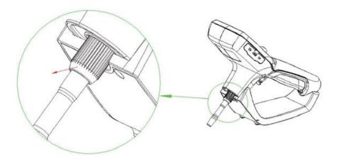
**Step 2:** Push the rubber sleeve upwards to remove replacement Tube.
