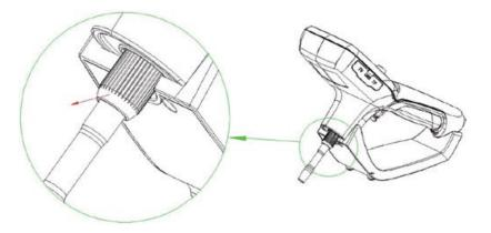
**Step 3:** After replacement Tube is inserted and aligned, tighten the locking nut on the back side of probe.
