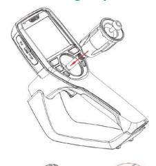
**Step 1:** Insert replacement Tube through the front side of scope.
