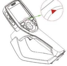
**Step 2:** Align the triangle located on the replacement Tube at top center
