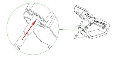
**Step 1:** Remove locking nut from the back side of the replacement Tube.
