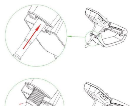
**Step 1:** Remove locking nut from the back side of the replacement Tube.
