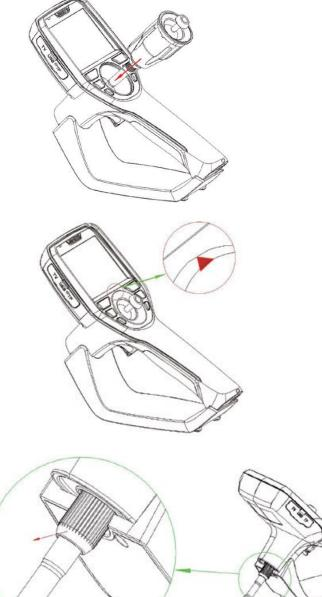
Step 1: Insert replacement Tube through the front side of scope.
