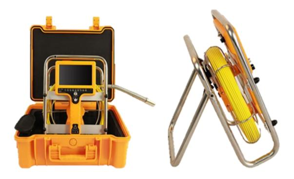
The RVI PC is a rugged Pipe Camera with a 5mm diameter fiberglass rod, 20 meter to 50 meter customizable lengths and interchangeable camera heads up to 28mm in diameter. Includes 12 levels of LED light control and a 7" monitor ready for video/ audio recording or still images. Equipment is enclosed in heavy duty ABS case.
