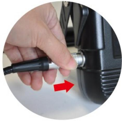
**Method:** Align the red dot on the tube with the red mark on the host, gently push the plug in. When you hear a “click”, the tube has been installed successfully.
