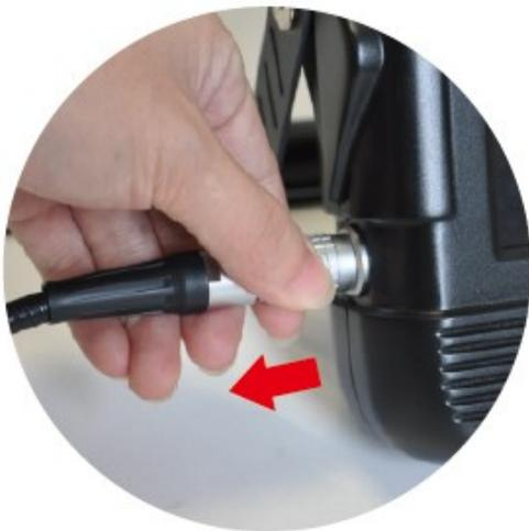
**Method:** Push out the locking ring at the connection of the tube plug, then pull out the tube from the host. Directly separate it from the host.
