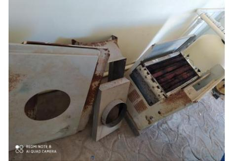
Most of the boilers are damaged and we have to replace them, some lack the pilot or are aberrated by the time of use, the heater pipes are pitted
