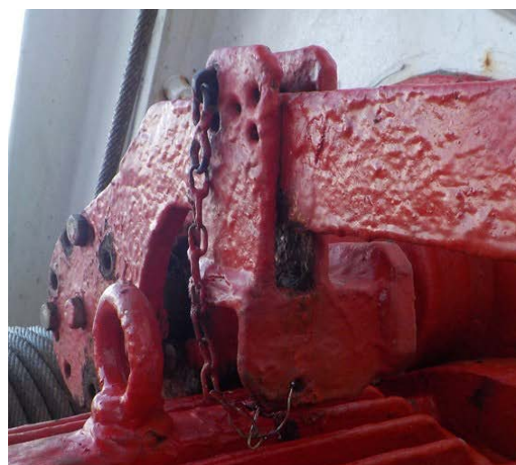
Example of correctly applied brake lever in a natural closed position
