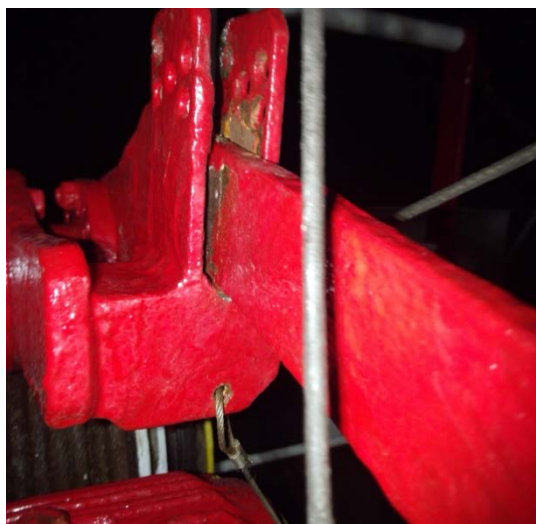
Example of incorrectly applied brake lever, forced closed against the holding bracket
