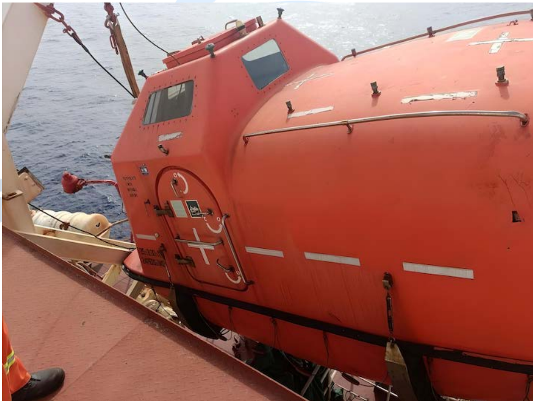
Figure 1: The port lifeboat suspended by FPD following opening of the aft hook due to a failed release gear cable. Note the angle of the boat indicating fwd hook is still properly engaged.
