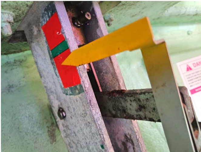
Figure 2: Aft hook indicator shows the hook is not properly reset. Despite which, the crew continued to force the system to close
