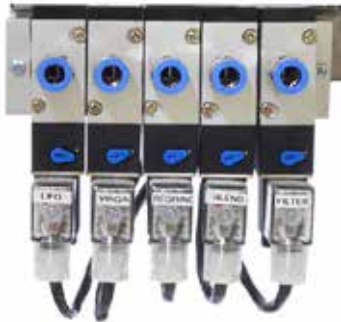
Valve manifold with spare valve and test buttons.
