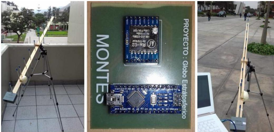
Figure 5.12: Pictures of the Yagi antenna
