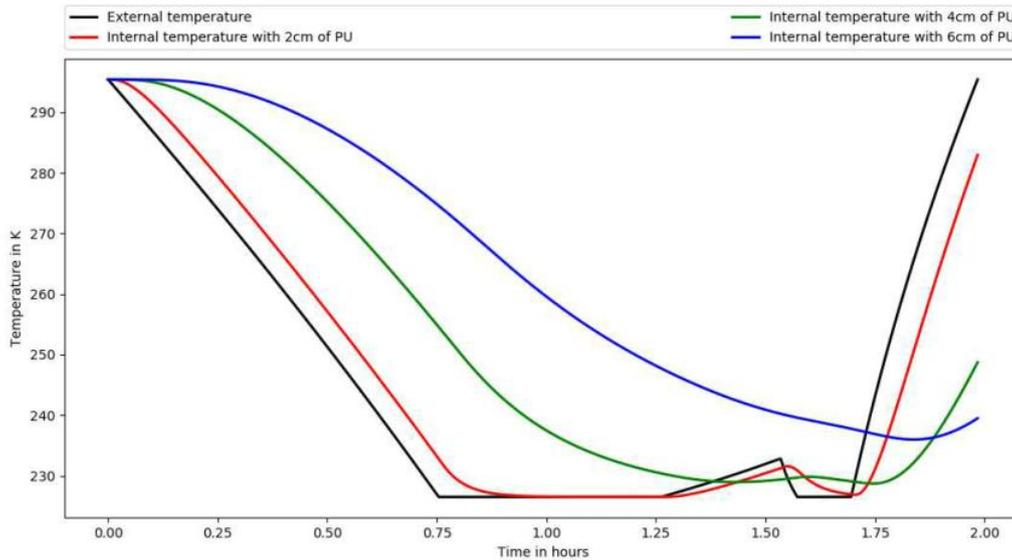
Figure 5.15: Evolution of the internal temperature with different thicknesses
