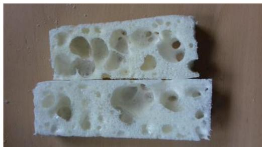
Figure 5.19: Internal structure of the PU in spray
