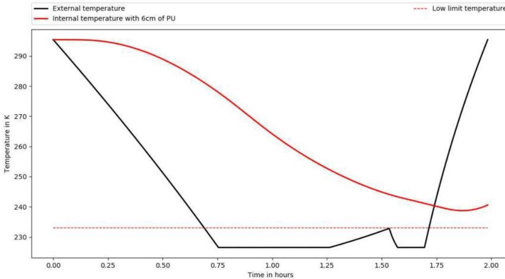
Figure 5.16: Evolution of the internal temperature with a 6 cm thickness
