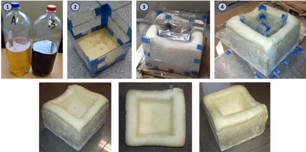
Figure 5.21: Moulding method with a mould in PVC and synthesized PU
