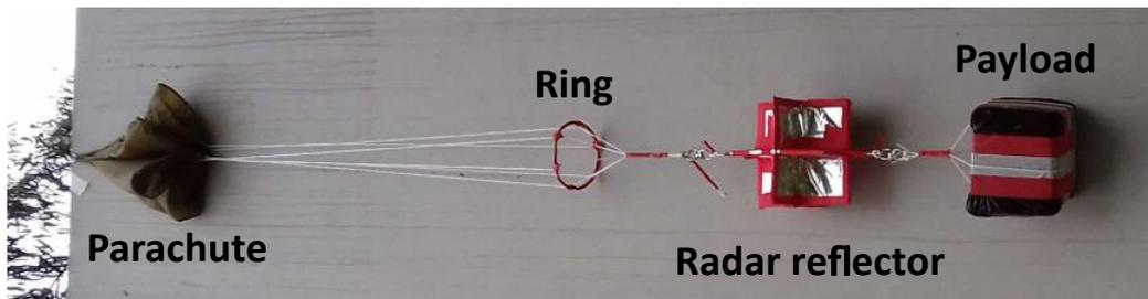
Figure 5.4: Picture of the chain of flight
