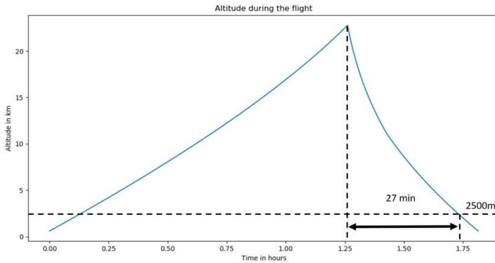
Figure 7.5: Vertical trajectory simulation and fall duration
