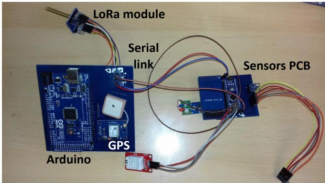
Figure 6.3: Picture of the sensors and the telemetry PCBs
