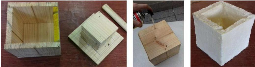
Figure 5.17: Moulding method with a mould in wood and PU in spray
