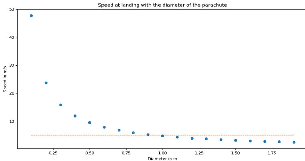
Figure 5.3: The speed at ground level with the diameter of the parachute
