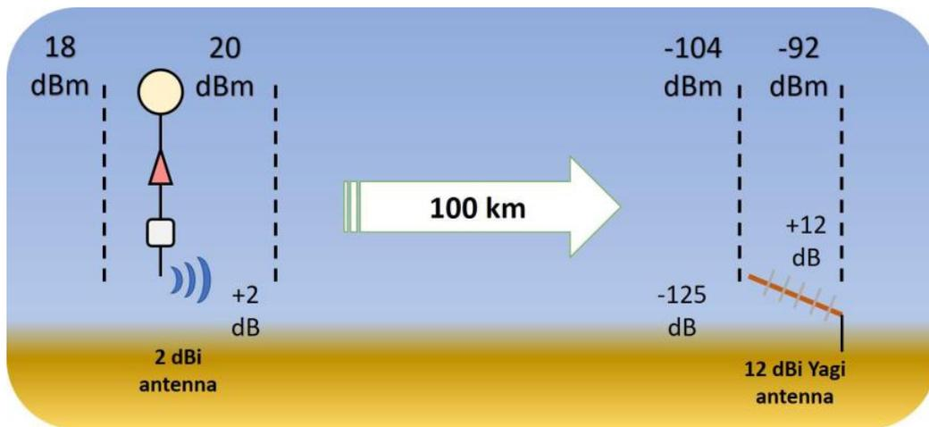
Figure 5.10: The link budget of the telemetry
