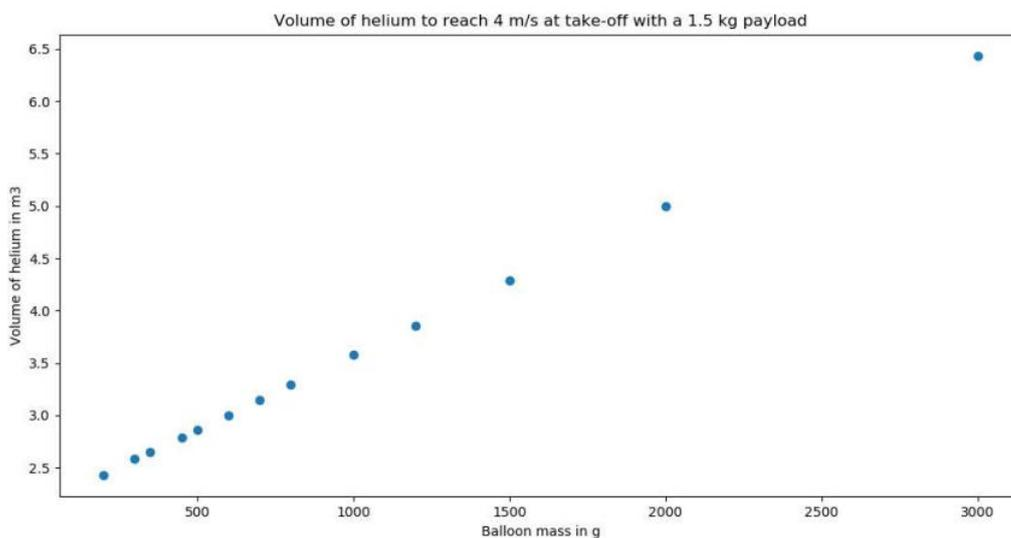
Figure 5.1: The required volume of helium to obtain a 4 m/s speed at launch
