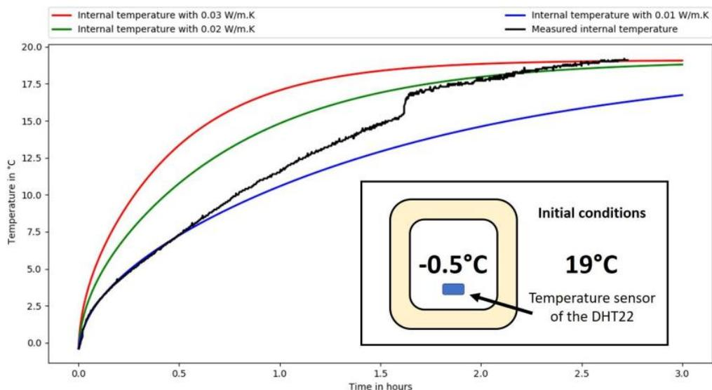
Figure 5.24: Evolution of temperature inside the box compared to simulations
