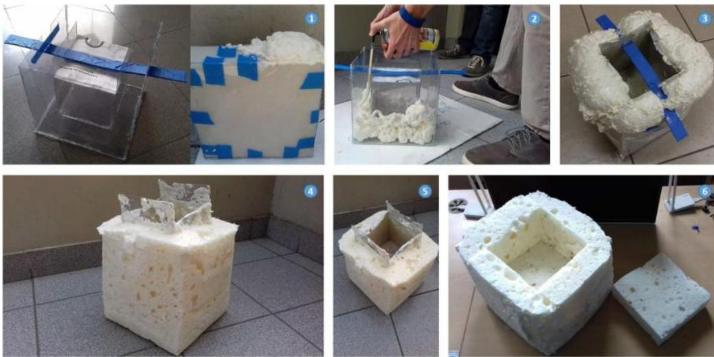
Figure 5.18: Moulding method with a mould in PVC and PU in spray
