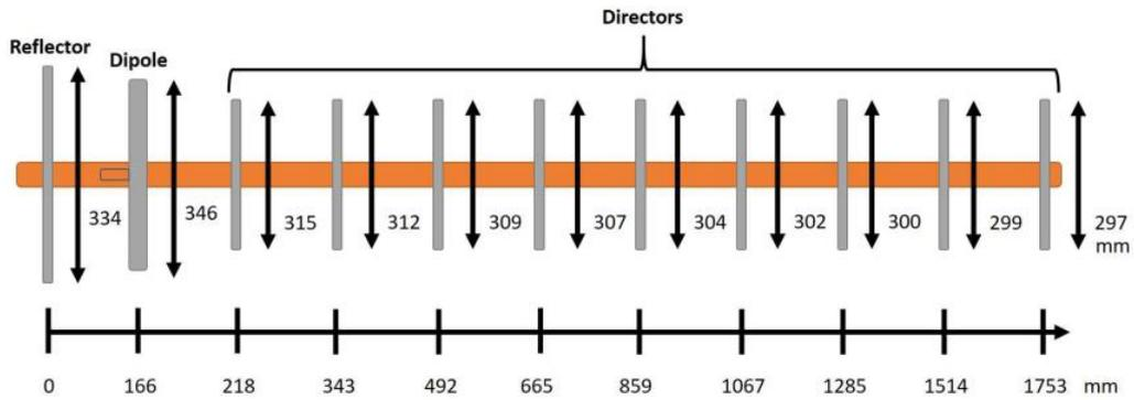
Figure 5.11: The dimensions of the Yagi antenna
