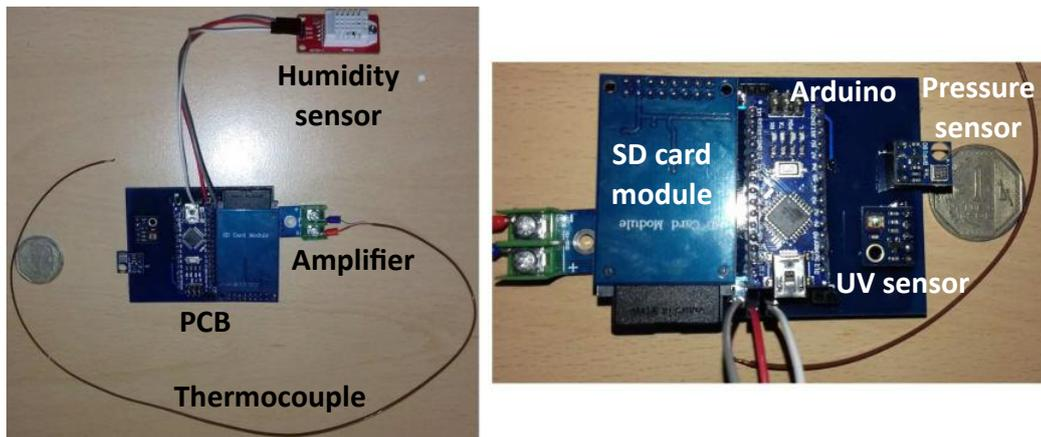
Figure 6.2: Picture of the sensors PCB
