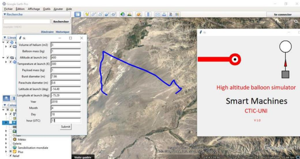
Figure 5.6: The developed trajectory simulator software
