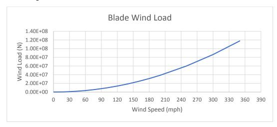
Figure 5– Wind load as a function of the wind speed in a 100m rotor.
