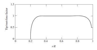
Figure 3 – Span-wise variation of combined tip/root-losses for a three-blade turbine optimized for a tip speed ratio of 6 and with a blade toot at 20% span (wind energy handbook).
