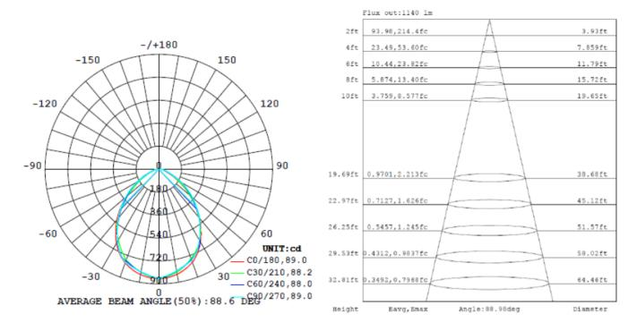
**8" DOWNLIGHT** - The curves indicate the illuminated area and the average illumination when the luminaire is at different distance.
