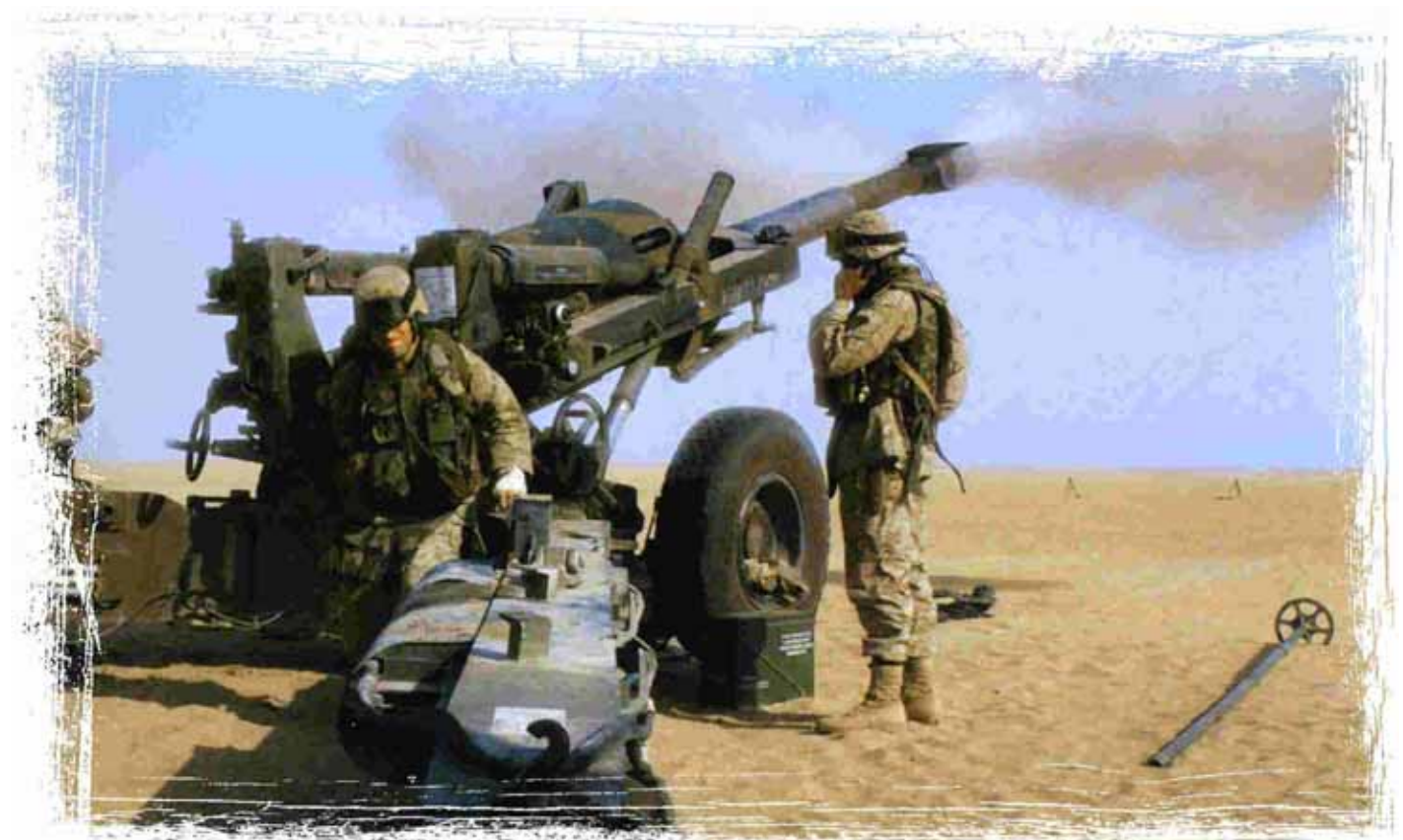
An M198 155mm Howitzer (range—approximately 18 miles) providing supporting fire for the 24th MEU somewhere in Iraq. [An excerpt from Semper Fi , by Col. H. Avery Chenoweth, USMCR (Retired) with Col. Brooke Nihart, USMC (Retired) and published by Main Street, a division of Sterling Publishing Co., Inc. of New York.]
