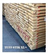
In a significant move towards improving kiln-drying efficiency and the quality of finished lumber, a growing number of kiln drying operations are upgrading from traditional and 'hybrid' wooden kiln sticks to the TUFF-STIK™ aluminum-alloy kiln sticks. This shift addresses longstanding challenges associated with wood kiln sticks, such as moisture retention, airflow obstruction, and the risk of catastrophic failure due to brittleness, while also delivering a fast return on investment (ROI).
