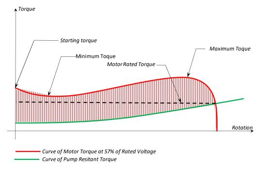
In the figure above are shown the motor curves with 57% of the rated voltage and the curve of the pump resistant torque. This condition corresponds to the motor with star-delta start.
