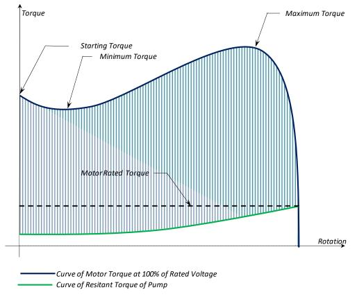
In the figure above are shown the curve of the motor with 100% of the nominal voltage and the curve of the pump's resistant torque. The hatched area represents the acceleration torque that defines the starting time of the set.
