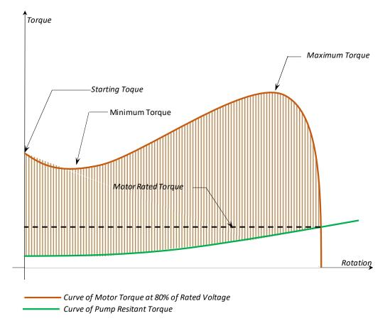
In the figure above are shown the motor curves with 80% of the nominal voltage and the curve of the pump resistant torque. The hatched area represents the acceleration torque that defines the starting time of the set. Note that the area corresponding to the acceleration torque is smaller than that of the previous figure and therefore the starting time will be longer.
