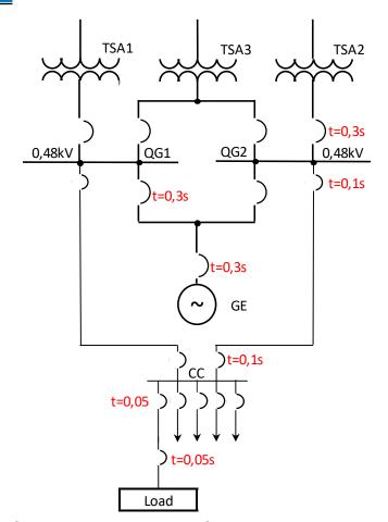
The actuation times of the protection devices of the same circuit are the same. For example, if a defect occurs in the load, the two circuit breakers, of the load and the load center (CC) output will open; if a defect occurs in the load panel feeder, only the load center (CC) output circuit breaker will open. The QG output protection and load center (CC) input protection will operate in the same way.
