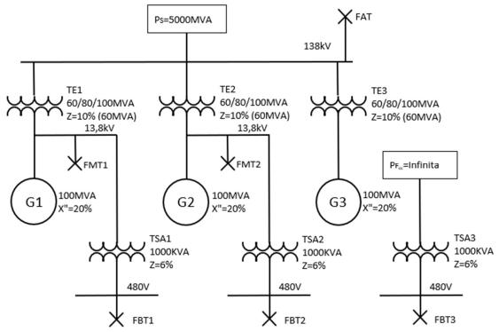
The calculation of the short circuit currents at the various points of the installation will be done using the MVA method. This method, by Monn H. Yuen, was published by the IEEE in 1974. The white paper, IT.EL.SA. CA.03 Short Circuit - Calculation of Currents, details this method for symmetrical three-phase short circuit currents and its concepts will be applied to the plant system, according to its information and indicated in the single-line diagram.
