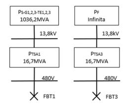
$$\begin{split} P_{S-G1,2,3-TE1,2,3} &= \frac{1}{\frac{1}{P_{S-G1,2,3-TE1,2,3}}} + \frac{1}{P_{TSA1}} = \frac{1}{\frac{1}{1036,2} + \frac{1}{16,7}} = 16,4MVA \\ I_{FBT1} &= \frac{16,4}{\sqrt{3}X0,48} = I_{FBT2} = 19,7kA \\ I_{FBT3} &= \frac{16,7}{\sqrt{3}X0,48} = I_{FBT2} = 20,1kA \end{split}$$
