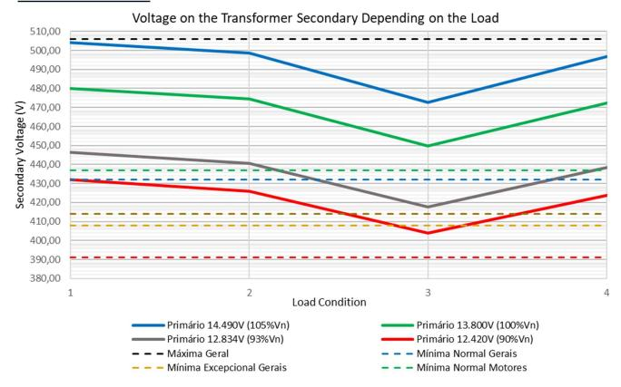
It is observed that if the voltage of the source of the primary transformer is within the appropriate voltage limit (from 93 to 105% of the nominal voltage) or precarious (from 90 to 93% of the nominal voltage), the system will operate normally, except during the start of the 100hp motor, when the voltage falls, transiently, below the minimum normal values of the general loads (480V, -10%) and minimum normal operation of the motors (460V, -5%).
