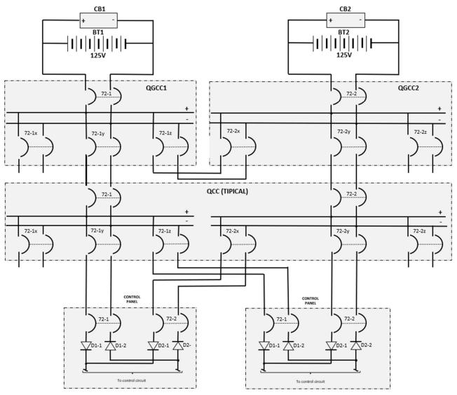
In the figure are indicated the battery sets (BT1 and BT2), chargers (CB1 and CB2), the general panels (QGCC1 and QGCC2), a typical direct current distribution panel (QCC) and two control panels that contain the circuits fed with the new configuration.
