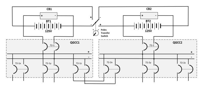
When performing the transfer of poles, one must be careful because if two defects have occurred to earth, one in each system and in different poles, in interrupting the interconnection to transfer of the interconnected poles, the situation that causes the overvoltage that one wants to avoid may occur.
