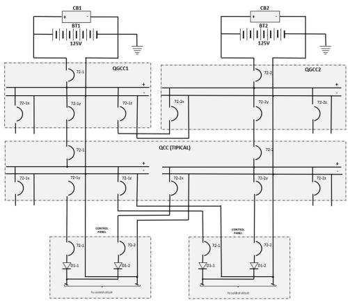
The following is the bifilar diagram of the alternate configuration (parallelism in DC distribution frames):
