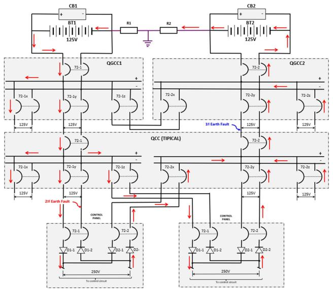
The resistors R1 and R2 represent the resistances of the faults to the ground, the value of which will depend on the severity of the failure. In the extreme condition, the voltage in the general panels (QGCC1 and QGCC2) and panels and distribution circuits represented by the QCC, will be 125V, but in all control panels and loads fed through the diodes, the voltage can reach 250V.
