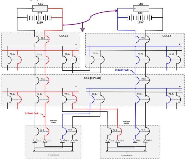
In the figure above it is indicated that the first ground failure occurs in the positive pole cable, of the panel feeder (QCC), coming from the general direct current panel (QGCC2). In this way, all the circuits of the positive pole of the system, powered by the charger and battery set (CB2 and BT2), indicated in blue color, will be at the same potential to the ground.
