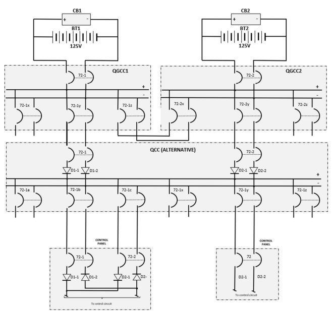
In the bifilar circuit above are indicated the battery sets (BT1 and BT2), chargers (CB1 and CB2), the general panels (QGCC1 and QGCC2), a typical direct current distribution board (QCC), a control panel containing the new configuration with dual power and a control panel without double power.
