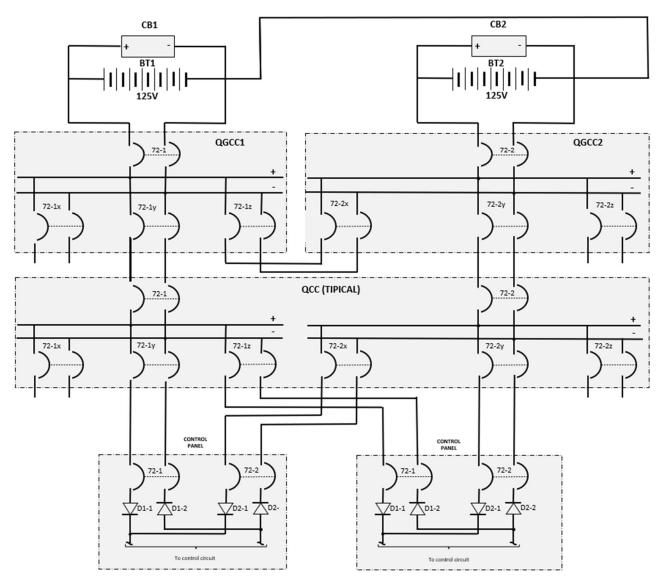
This solution for the alternative configuration, interconnecting the negative poles of the battery charger assemblies, is represented in the bifilar diagram of the following figure:
