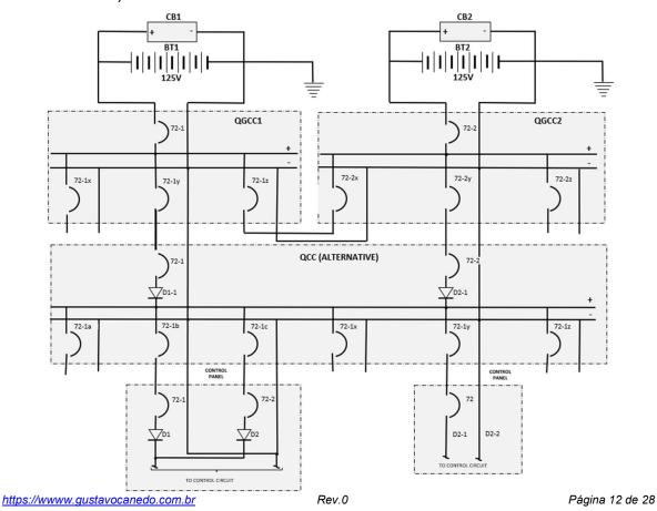
In this solution, any defect to the earth will cause the faulty circuit to shut down. If this solution is adopted, it is not necessary for the circuit breakers to be bipolar, as the system is grounded.
