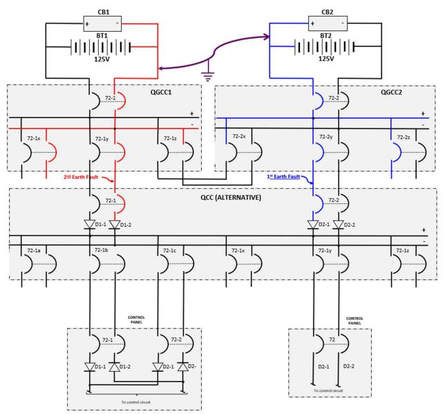
In the figure above it is indicated that the first ground failure occurs in the positive pole cable, of the panel feeder (QCC), coming from the general direct current panel (QGCC2). In this way, all the circuits of the positive pole of the system, powered by the charger and battery set (CB2 and BT2), indicated in blue color, will be at the same potential to the ground.
