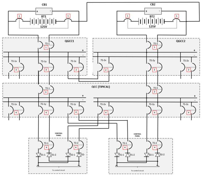
The selectivity between battery protection (1) and the input of the general QGCC frame (1) can be omitted. If a defect occurs in the QGCC bar the panel and battery input protections should act and lack of selectivity will not change the operating condition of the installation. If a defect occurs in the QGCC feeder, only the battery protection should act. The battery charger has its own protection that does not need to enter the study.
