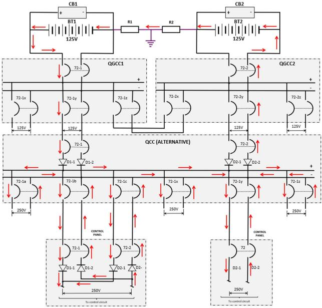
The resistors R1 and R2 represent the resistances of the faults to the ground, the value of which will depend on the severity of the failure. In the extreme condition, the voltage in the general frames (QGCC1 and QGCC2) will be 125V, but in all switchboards and their loads it can reach 250V.
