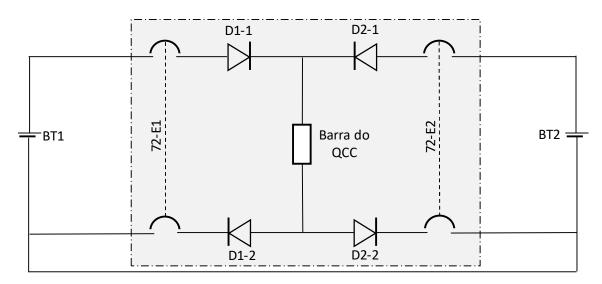
The supply current of the panel can occur through the diodes D1-1 or D2-1, but the return may not necessarily occur by the diodes D1-2 or D2-2, respectively. Therefore, before opening an input circuit breaker one must be sure of the integrity of the diodes of the other source.
