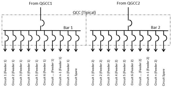
In the above configuration the distribution panels can have two direct current bars or, preferably, be formed by two independent sections, each powered by one of the direct current sources of the plant. From the panels are made the feeds of the direct current loads of the plant, with a feeder of each bar.
