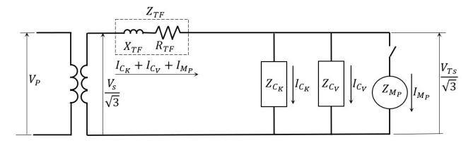
The figure above represents the circuit of a transformer that feeds a load set composed of loads with constant power, loads with variable power and starting of motors.
