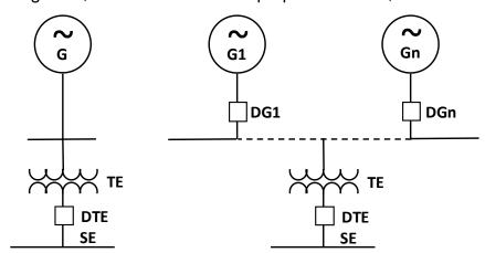
In the case of only one generator unit by step-up transformer, synchronization of the unit with the substation is done through the DTE circuit breaker. In the case of more than one generator unit by step-up transformer, the synchronization of the first unit with the substation is done through the DTE circuit breaker and the other units are synchronized, in the generation bar, through the circuit breakers of the respective units DG1, ..., DGn.
