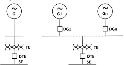
Although there is more than one unit per step-up transformer, synchronization of the first unit occurs as if the others did not exist, that is, synchronization of the first unit is always done through the DTE circuit breaker.
