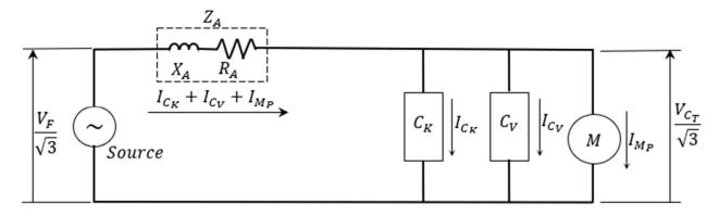
The circuit figure above represents the circuit at the instant the loads are turned on.
