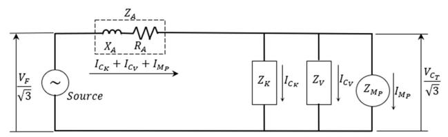
The figure above represents the circuit of a feeder that feeds a load composed of load with constant power, load with variable power and starting of motor(s).
