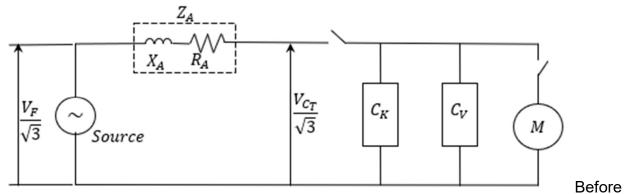
the load is switched on, the voltage at the terminal of the feeder circuit  $V_{C_T}$  will be equal to the voltage of the source  $V_F$ .
