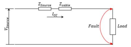
To simplify the calculations, it will be considered that the impedance of the source will be the reactance, calculated based on the short circuit power of the source. Like this:
