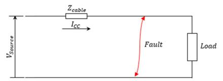
Considering that the short-circuit power at the source is infinite, which will not significantly change the result, we have:
