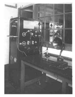
The RT transmitter was Marconi Type XMC 1 Telephone Set and was in fact a 500W transceiver. Initially it was used for message traffic only but in 1937 the first ever telephone 'link call' was made when a trawler was connected to his company office through the telephone system. It was a fairly crude simplex system transmitting on 163 metres and receiving on 139 metres with all TX & RX levels being set by hand.
