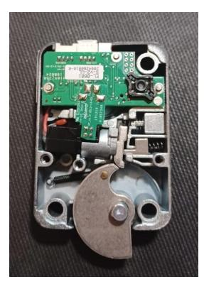
Let's take for example a Securam lock mounted VD, with the flat of the swingbolt to your left.
