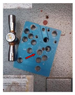
This is how the template would look, mounted for a VD lock with the flat to your left. You would attach your MiniRig to the LG hole.
