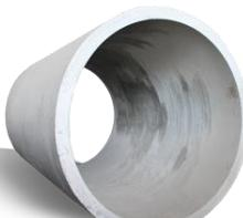
We provide an extensive range of pipes from nominal diameter of 300mm up to 3000mm. All reinforced concrete pipes from Bilcon Industries can be produced with grade 40 concrete or higher based on your requirements. To fulfil the requirements of a modern, durable wastewater drainage system, we also provide the options of using Ordinary Portland Cement (OPC), Sulphate-Resisting Cement (SRC), as well as the Calcium Aluminate Cement (CAC).
