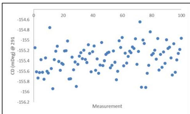
**Fig. 1. Consecutive measurements in wells A10 & F2 of (-) CSA as a function of measurement.** Successive measurements of 200 µl of (-) CSA (Sigma) at 1 mg/ml in wells #A10 & #F2 of a solid fused silica 96 well plate (Hellma) taken at 291 nm. Data was collected with no effort to minimize evaporation (samples were not protected with an optically clear cover) or reduce the noise (data were collected with the shortest integration times possible) at a room temperature of 25°C.
