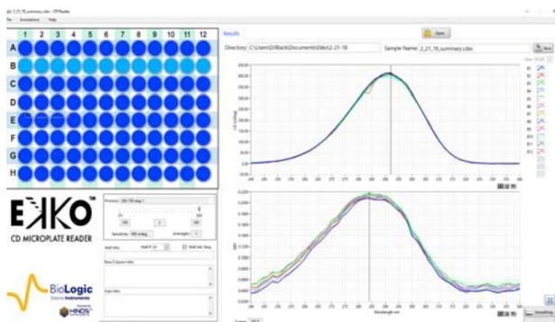
**Fig. 3. Raw CD spectra of CSA.** The CD spectra of 200 µl H<sub>2</sub>O & (+) CSA (Sigma) at 3 mg/ml in wells #A1-H12 of a solid fused silica 96 well plate with black sidewalls (Hellma) from 240 - 340 nm were taken. Raw data was collected with no effort to minimize the noise or evaporation at a room temperature of 25°C. Representative data from cells B1-B12 are shown.
