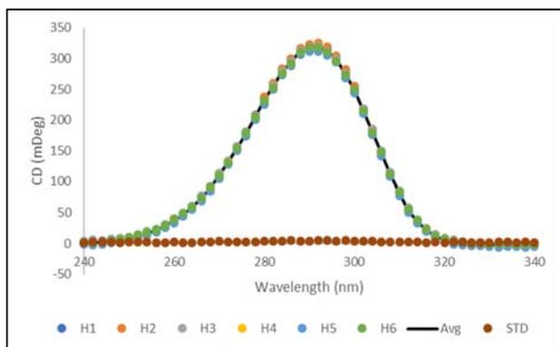
**Fig. 5. Raw CD spectra of CSA from the final row of wells of an unskilled technician.** The CD spectra of 200  $\mu$ l (+) CSA (Sigma) at 1 mg/ml in wells #H1-H6 of a solid silica bottom 96 well plate with black sidewalls (Porvair) from 240 - 340 nm were taken. Raw data were collected with no effort to minimize the noise or evaporation at a room temperature of 25°C. Wells H1-H6 are shown in addition to the mean and standard deviation of those six.
