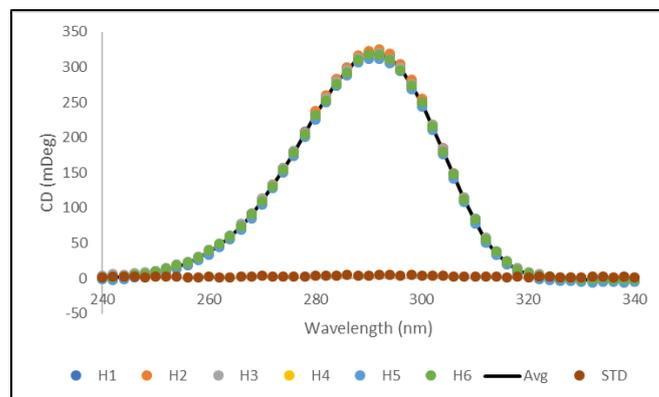
**Fig. 4. Raw CD spectra of CSA from the final row of wells of an unskilled technician.** The CD spectra of 200 µl (+) CSA (Sigma) at 1 mg/ml in wells #A1-H12 of a solid silica bottom 96 well plate with black sidewalls (Porvair) from 240 - 340 nm were taken. Raw data were collected with no efforts to minimize the noise or evaporation at a room temperature of 25°C. Wells H1-H6 are shown in addition to the mean and standard deviation of those six.
