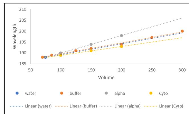
**Fig. 6. Cut Off Wavelength as a Function of Volume.** Replots of the cut off wavelength as a function of volume for H<sub>2</sub>O, K<sub>2</sub>PO<sub>4</sub> (10 mM, pH 7.4 Sigma),  $\alpha$ -lactoglobulin (40  $\mu$ g/ml Sigma) and Cytochrome C (40  $\mu$ g/ml Sigma). Each point data point represents the STD of  $n \geq 12$  individual spectra.
