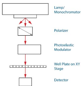
The EKKO™ CD Microplate Reader is a vertical CD spectrometer that turns the measuring light beam from the horizontal direction to vertical allowing for
