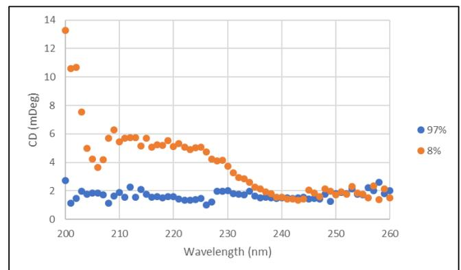
**Fig. 8. Standard Deviation as a function of Wavelength for the Averaged CD spectra for the different Solid Fused Silica Well Plates (Hellma).** The standard deviation of the n=30 CD spectrum of 200  $\mu$ l of Insulin (Sigma) at 50  $\mu$ g/ml in wells C2-E11 of two solid fused silica 96 well plates (Hellma) with different optical characteristics were recorded at 25°C with an integration time of 1 sec/nm.
