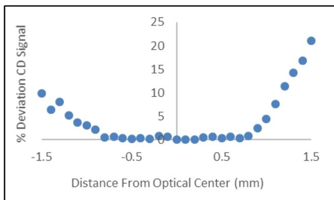
**Fig. 3. % signal deviation as a function of distance from the optical center of the well.** 200 µl of CSA (Sigma) at 0.2 mg/ml was in well #F10 of a solid fused silica 96 well plate (Hellma). The CD signal was collected for 30 displacements of the beam path along the X-axis at 290 nm. Each position was 0.1 mm incrementally further away from the optical center of the well. Data is plotted as the % deviation from the mean.
