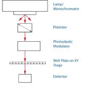
The EKKO<sup>™</sup> CD Microplate Reader is a vertical CD spectrometer that turns the measuring light beam from the horizontal direction to vertical allowing for
