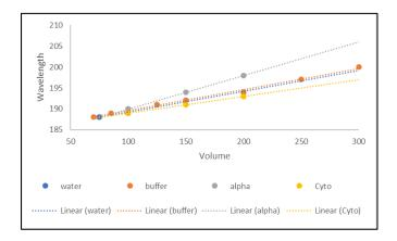
Fig. 6. Cut Off Wavelength as a Function of Volume. Replots of the cut off wavelength as a function of volume for H<sub>2</sub>0, K<sub>2</sub>PO<sub>4</sub> (10 mM, pH 7.4 Sigma),  $\alpha$ -lactoglobulin (40 µg/ml Sigma) and Cytochrome C (40 µg/ml Sigma). Each point data point represents the STD of n ≥ 12 individual spectra.
