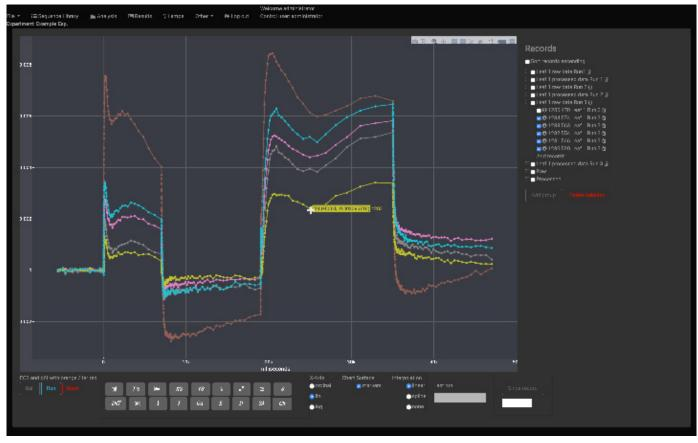
Collected data is displayed on an interactive screen. Scaling functions are click and drag. Data sets can be grouped for easier selection Moving the cursor over a trace shows point by point detail.
