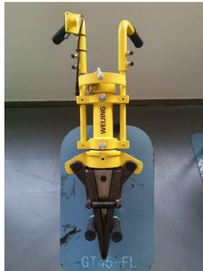
Vertical wedge for ground level degating
