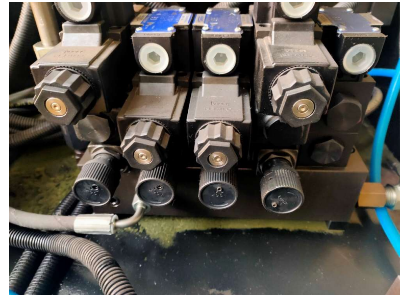
Right Image Solenoid valves to control hydraulic cylinder & vane motor working.
